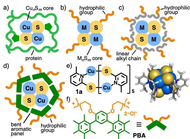
Fig. 1 Preparation of aqueous  $\text{Cu}_n\text{S}_m$  or  $\text{M}_n\text{S}_m$  cluster-based solutions, using (a) a protein cavity, (b) hydrophilic thiol ligands and (c) an alkyl micelle (except for  $\text{M} = \text{Cu}$ ), and (d) an aromatic micelle (this work). (e)  $\text{Cu}_6\text{S}_6$  cluster **1a** and its crystal structure.<sup>14,15</sup> (f) Bent aromatic amphiphile PBA.
