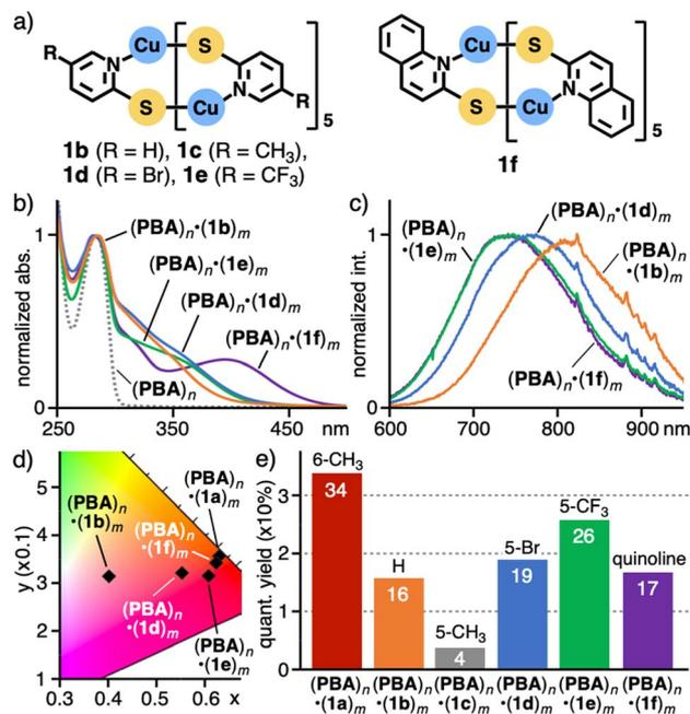
Fig. 4 (a)  $Cu_6S_6$  clusters  $1b-f$  with various substituents. (b) UV-visible spectra ( $H_2O$ , r.t., 1.0 mM based on  $PBA$ ) of host-guest complexes  $(PBA)_n \cdot (1b)$  or  $1b-f)_m$  and (c) their emission spectra ( $\lambda_{ex} = 320$  nm). (d) CIE diagram ( $H_2O$ , r.t.,  $\lambda_{ex} = 320$  nm) of  $(PBA)_n \cdot (1a-f)_m$  in water and (e) their emission quantum yields.
