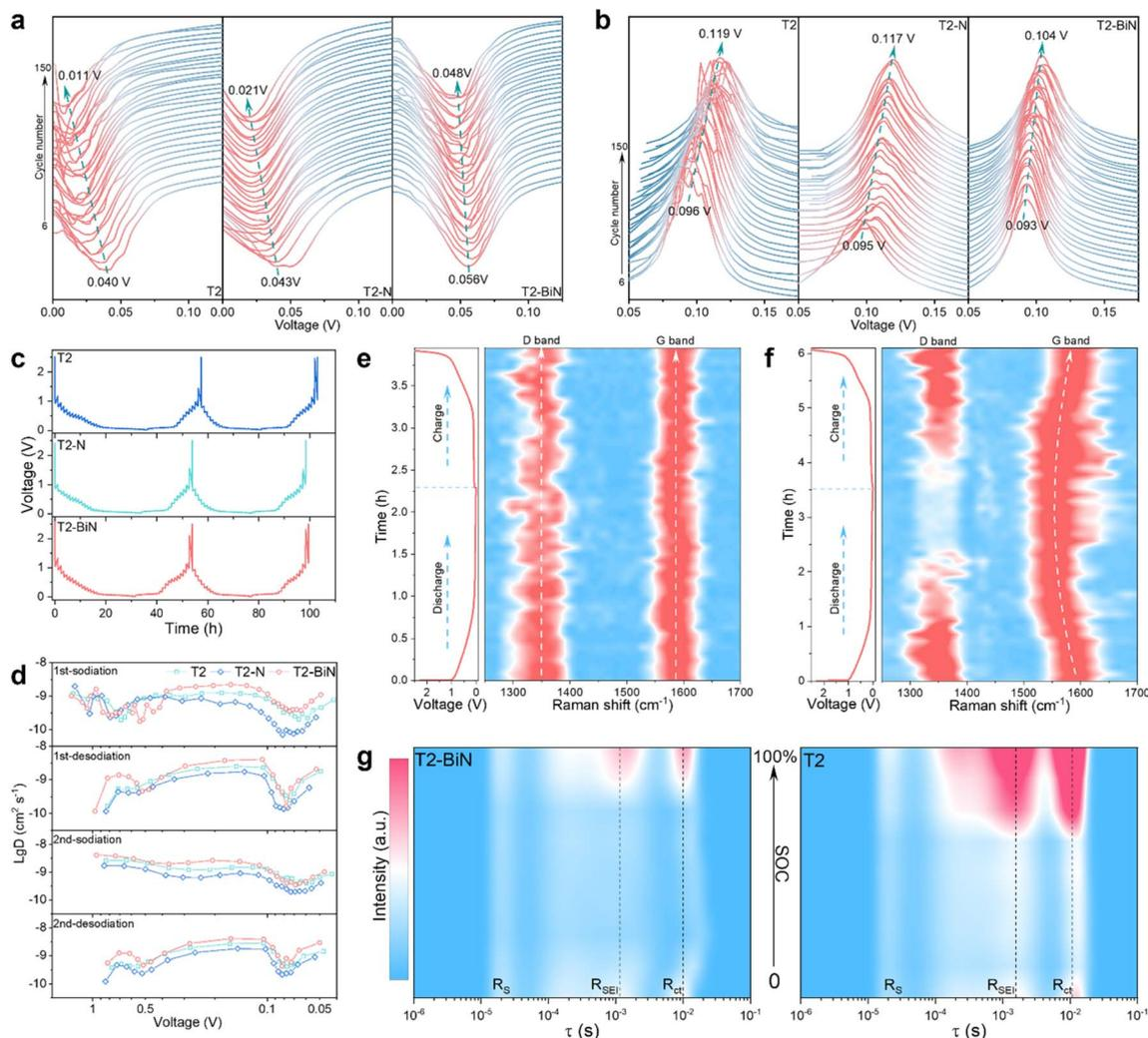
Fig. 4 Reaction kinetics and sodium-storage mechanism of T2 and T2-BiN. (a) The  $dQ/dV$  profiles showing the dynamic evolution of the reduction peak (a) and oxidation peak (b) during the cycling tests; (c) GITT profiles of the first two cycles and (d) the corresponding  $\text{Na}^+$  diffusion coefficients; *in situ* Raman of T2 (e) and T2-BiN (f) showing the evolution of D and G band; (g) 2D DRT profiles of T2 and T2-BiN anodes during the first discharging process.
