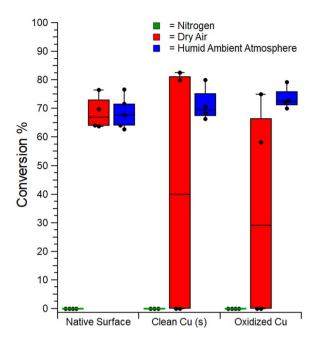
Fig. 3 Box plots showing the mechanocatalytic performance of the copper catalysed p-toluenesulfonamide and n-butyl isocyanate coupling reaction with Cu-BBs of differently prepared surfaces under different atmospheric conditions. Milling parameters: 25 mL stainless steel hermetically sealed jars, Cu-BBs (20 count), 1.25 mmol scale, 30 Hz, 2 h.
