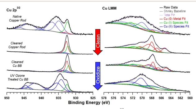
Fig. 2 X-ray photoelectron spectroscopy (XPS) measurements of Cu LMM and  $Cu(2p^{3/2})$  peaks and associated fits with different copper metal pre-treatments demonstrating capacity to control metal surface composition.
