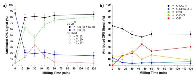
Fig. 4 XPS surface area coverage measurements of the Cu-BBs surface (a) of  $Cu(2p^{3/2})$  and LMM peaks and (b) C(1s) peaks as a function of milling time. Milling parameters: stainless steel hermetically sealed jars, Cu-BBs (20 count), 30 Hz, 2 h, ambient atmosphere.
