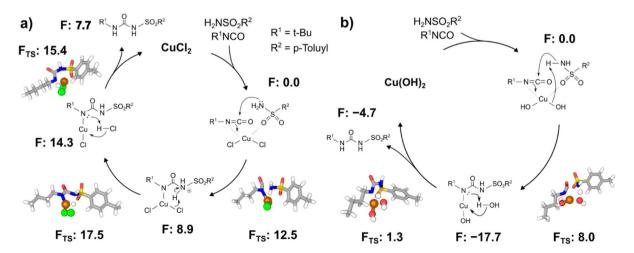
Fig. 7 Proposed mechanisms for tolbutamide formation with (a)  $CuCl_2$  and (b)  $Cu(OH)_2$  as the active catalyst. Free energies are shown in kcal  $mol^{-1}$  from DFT.
