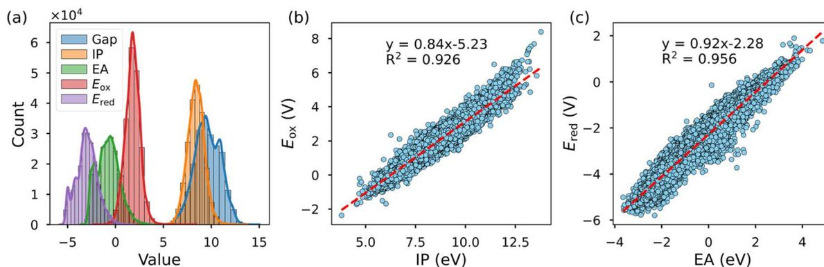
Fig. 5 (a) Histogram of the distribution of five properties predicted by the AIMNet2 model on the entire dataset. (b) Correlation between IP and  $E_{ox}$ . (c) Correlation between EA and  $E_{red}$ .
