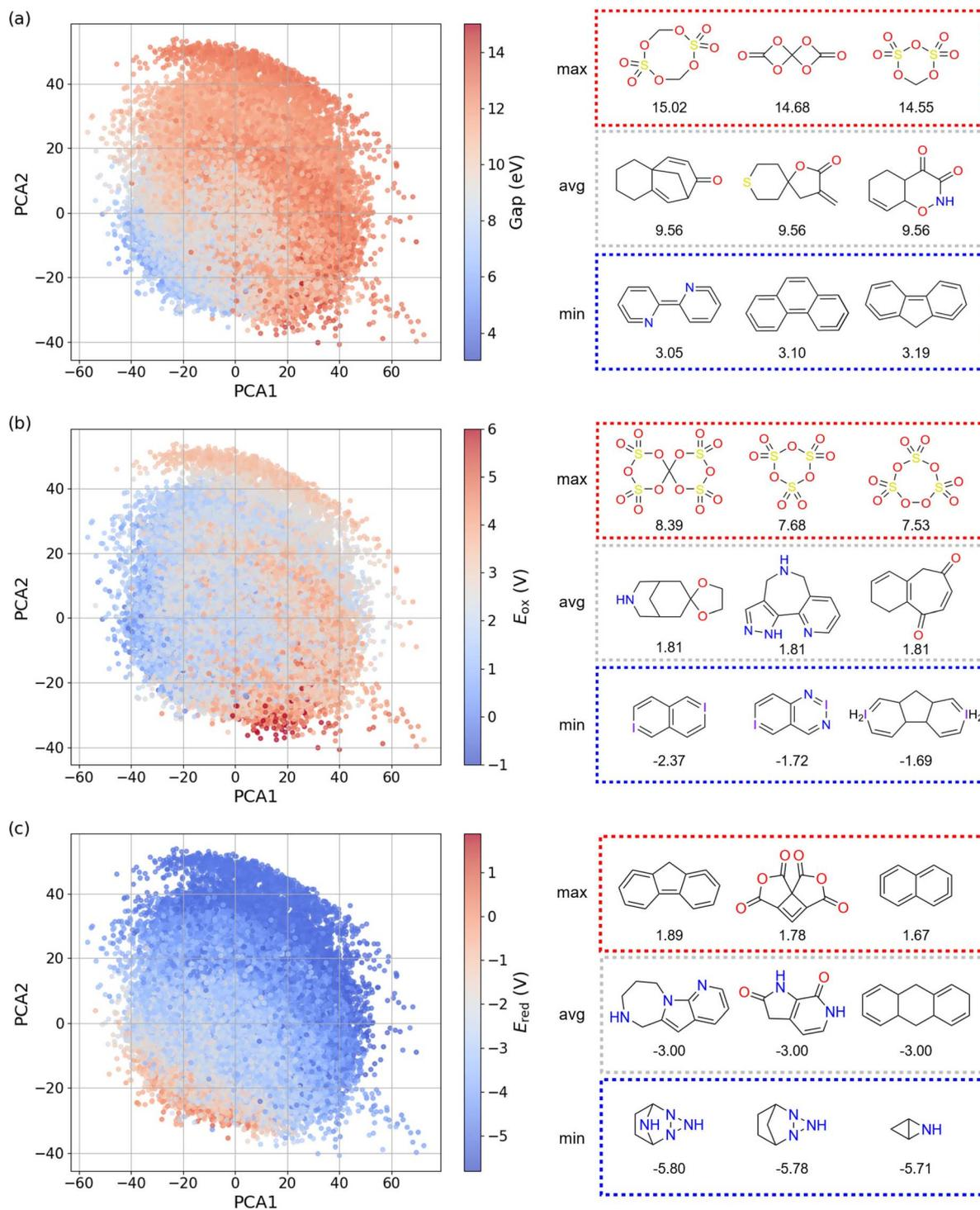
Fig. 6 PCA projection of the AIMNet2 molecular embeddings. (a) Points color-coded by HOMO–LUMO gap (eV). (b) Points color-coded by  $E_{\text{ox}}$  (V). (c) Points color-coded by  $E_{\text{red}}$  (V). The three molecules with the highest, lowest, and closest-to-average values for each property are highlighted on the right panel.
