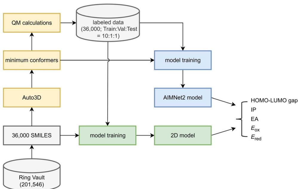
Fig. 2 Workflow of data preparation and model training.
