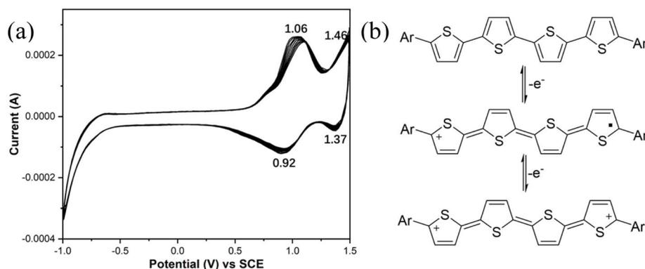
Fig. 14 (a) Cyclic voltammogram of 4T in  $0.1 \text{ M Bu}_4\text{NPF}_6/\text{acetonitrile}$  electrolyte with a scan rate of  $100 \text{ mV s}^{-1}$  (cycle 10 times); (b) the chemical structure change of oligothiophene in the redox process.
