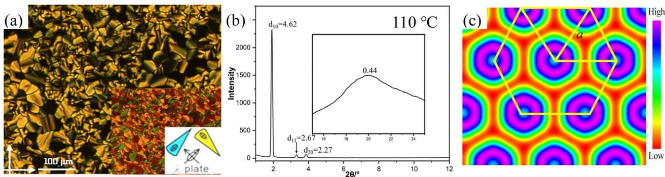
Fig. 1 (a) The optical texture of 2T at 110 °C; the inset shows the textures with an additional  $\lambda$ -retarder plate. (b) SAXS pattern of the  $\text{Col}_{\text{hex}}/p6mm$  phase of 2T at specific temperatures; the inset shows the corresponding WAXS pattern. (c) Reconstructed ED map of the  $\text{Col}_{\text{hex}}/p6mm$  phase showing a hexagonal plane with aromatic cores and alkyl chains.
