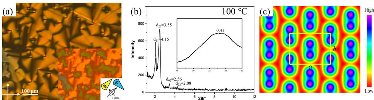
Fig. 3 (a) The optical texture of **5T** at 100 °C; the inset shows the texture with an additional  $\lambda$ -retarder plate. (b) SAXS pattern of the Col<sub>rec</sub>/c2mm phase of **5T** at specific temperatures; the inset shows the corresponding WAXS pattern. (c) Reconstructed ED map of the Col<sub>rec</sub>/c2mm phase showing a rectangular plane with aromatic cores and alkyl chains.
