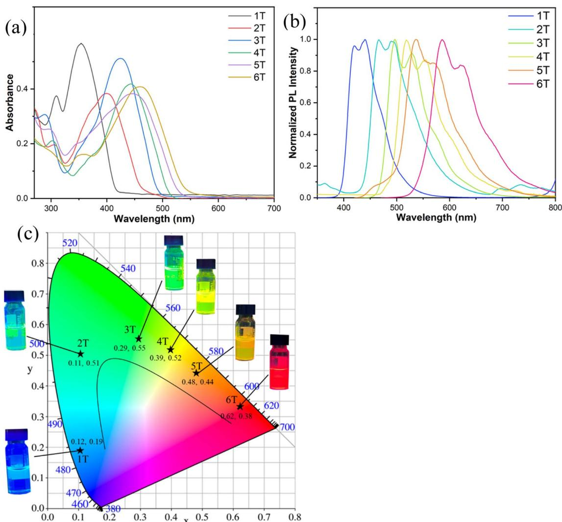
Fig. 10 Spectral information of  $nT$  in DCM solution ( $10^{-5}$  M). (a) Absorption spectra; (b) PL spectra; (c) chromaticity coordinate chart of the six compounds. The insets show the photoluminescence images (365 nm) of six compounds in DCM.
