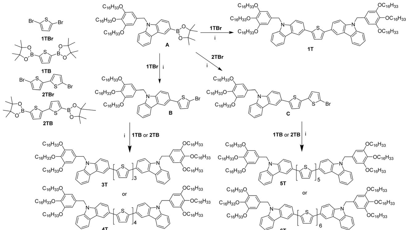
Scheme 2 Synthesis of  $nT$ . Reagents and conditions:  $\text{Pd}(\text{PPh}_3)_4$ ,  $\text{K}_2\text{CO}_3$ ,  $\text{H}_2\text{O}$ , THF,  $\text{N}_2$ ,  $80^\circ\text{C}$ , 12 h.
