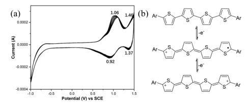
Fig. 14 (a) Cyclic voltammogram of 4T in  $0.1 \, M \, Bu_4 NPF_6$ /acetonitrile electrolyte with a scan rate of 100 mV s<sup>-1</sup> (cycle 10 times); (b) the chemical structure change of oligothiophene in the redox process.
