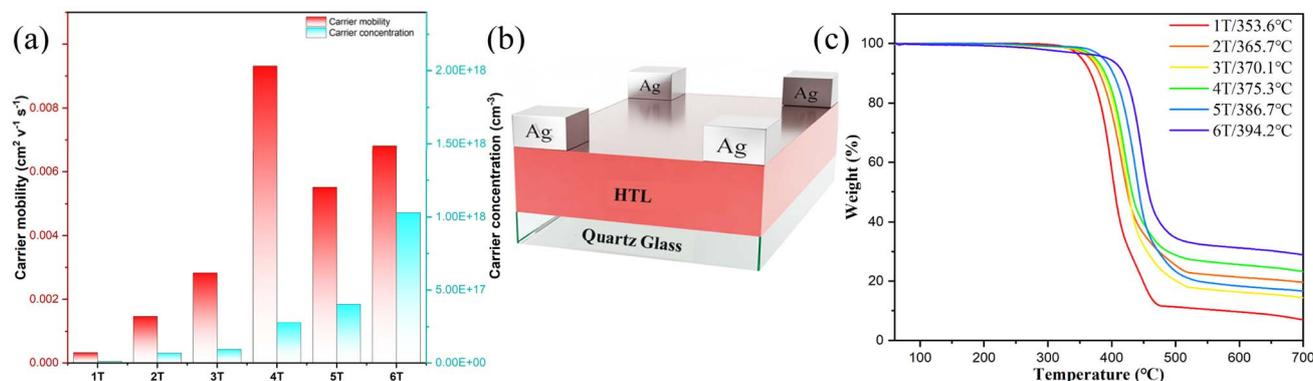
Fig. 15 (a) Carrier mobility of *n*T HTLs; (b) Hall device structure; (c) TGA curves of **1T–6T**. The measurements were performed under a nitrogen atmosphere, with heating rates of  $10 \text{ }^\circ\text{C min}^{-1}$ .
