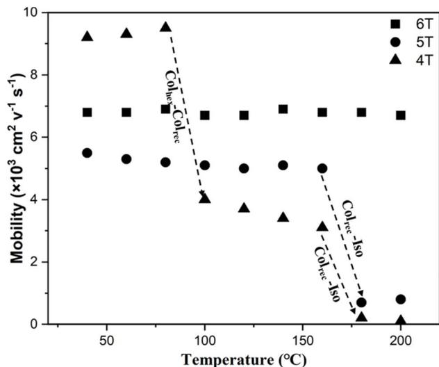
Fig. 17 Temperature dependence of carrier mobility. The dashed lines denote the phase transitions.
