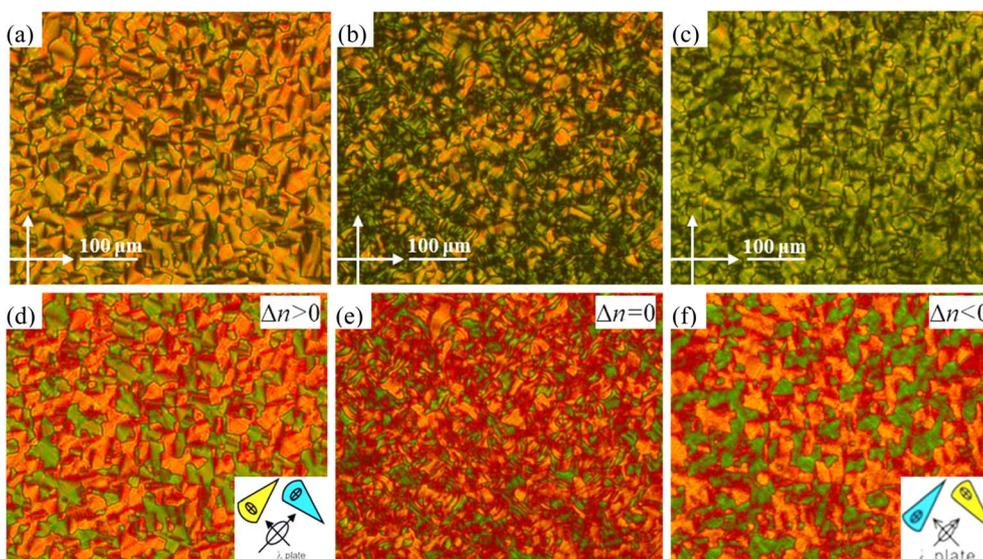
Fig. 6 (a–c) The optical textures of 4T are shown between crossed polarizers when it cools from  $Col_{rec}$  (155 °C) via a transient phase (89 °C) to the  $Col_{hex}/p6mm$  phase (87 °C); the textures with an additional  $\lambda$ -retarder plate are shown in (d–f).
