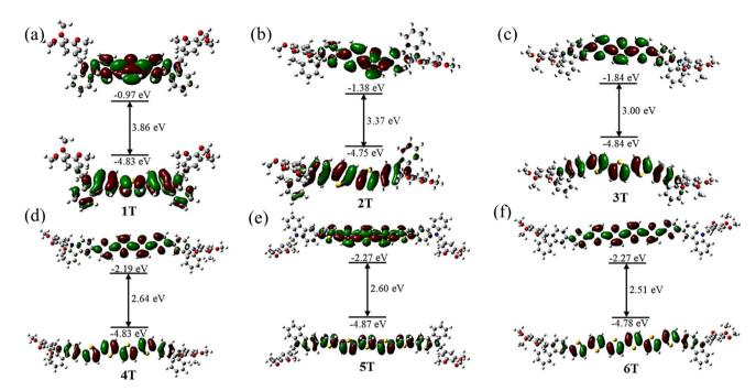
Fig. 13 Electron density distribution and energy levels of the HOMO and LUMO for nT (the long alkyl chains have been replaced by methyl).
