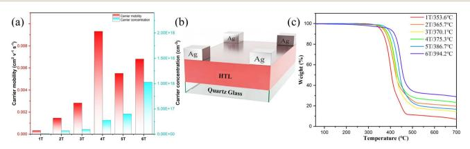
Fig. 15 (a) Carrier mobility of nT HTLs; (b) Hall device structure; (c) TGA curves of 1T-6T. The measurements were performed under a nitrogen atmosphere, with heating rates of 10 °C min<sup>-1</sup>.
