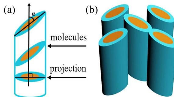
Fig. 4 Molecular tilted stacking model of the Col<sub>rec</sub>/c2mm phase.
