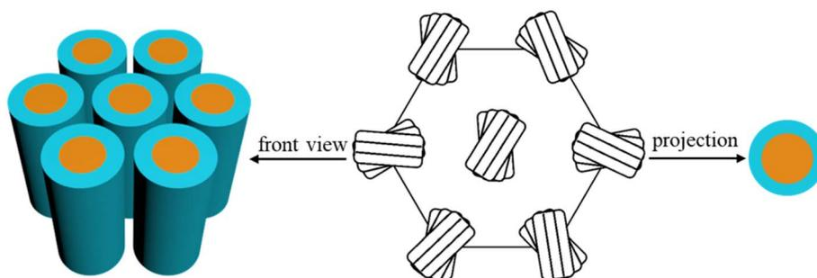
Fig. 2 Molecular stacking model of the  $\text{Col}_{\text{hex}}/p6mm$  phase.
