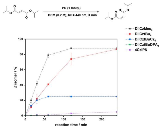
Fig. 5 Reaction progression for the  $E/Z$  isomerization of diisopropyl fumarate under  $N_2$ .  $E/Z$  ratios are given in %  $Z$  isomer after  $x$  minutes irradiated at 440 nm. Diisopropyl fumarate (0.2 mmol) in DCM (0.2 M) and PC (1 mol%).  $E/Z$  ratios were determined by  $^1H$  NMR spectroscopy.
