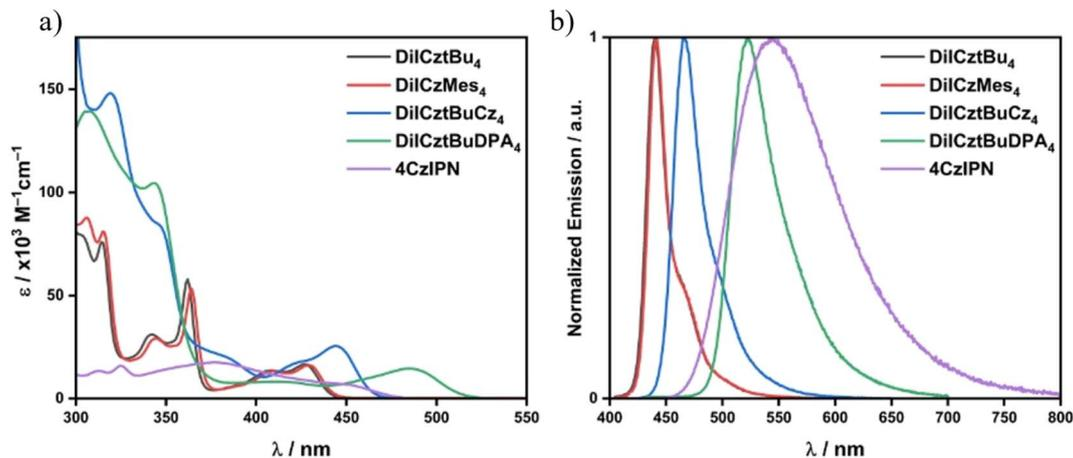
Fig. 3 (a) Absorption and (b) steady-state PL spectra in DCM of DiICztBu<sub>4</sub> ( $\lambda_{\text{exc}} = 340$  nm), DiICzMes<sub>4</sub> ( $\lambda_{\text{exc}} = 380$  nm), DiICztBuCz<sub>4</sub> ( $\lambda_{\text{exc}} = 340$  nm), DiICztBuDPA<sub>4</sub> ( $\lambda_{\text{exc}} = 400$  nm), and 4CzIPN ( $\lambda_{\text{exc}} = 378$  nm).
