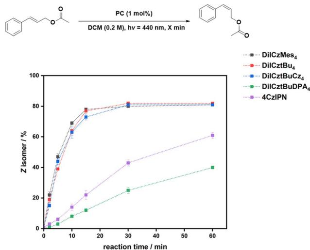
Fig. 4 Reaction progression for the *E/Z* isomerization of cinnamyl acetate in air unless otherwise noted. *E/Z* ratios are given in % *Z* isomer after *x* minutes ( $\lambda_{\text{exc}} = 440 \text{ nm}$ ). Cinnamyl acetate (0.2 mmol) in DCM (0.2 M) and PC (1 mol%). *E/Z* ratios were determined by  $^1\text{H}$  NMR spectroscopy. Reactions with **DiICztBuDPA<sub>4</sub>** as the PC were performed under  $\text{N}_2$ .
