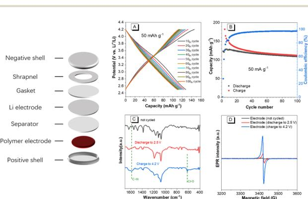
Fig. 5 Schematic illustration of the battery assembly (left) (A) the charge–discharge curves and (B) cycling stability at 50 mA h g<sup>−1</sup> of PIV cathode, respectively. (C) FT-IR spectra and (D) electron paramagnetic resonance (EPR) spectra of the PIV cathode in different states, respectively.
