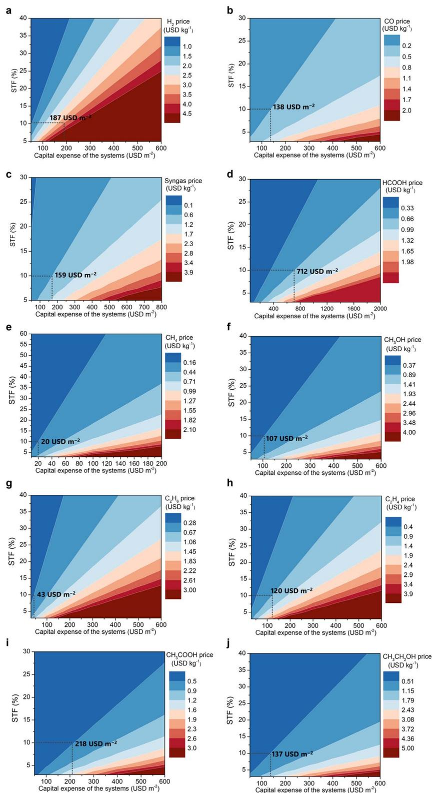
Fig. 5 Contour plots of the attainable price of (a) hydrogen (H<sub>2</sub>) and various CO<sub>2</sub>RR products: (b) carbon monoxide (CO), (c) syngas (H<sub>2</sub>/CO = 2), (d) formic acid (HCOOH), (e) methane (CH<sub>4</sub>), (f) methanol (CH<sub>3</sub>OH), (g) ethane (C<sub>2</sub>H<sub>6</sub>), (h) ethylene (C<sub>2</sub>H<sub>4</sub>), (i) acetic acid (CH<sub>3</sub>COOH) and (j) ethanol (CH<sub>3</sub>CH<sub>2</sub>OH) as a function of STF and capital expense for the system.
