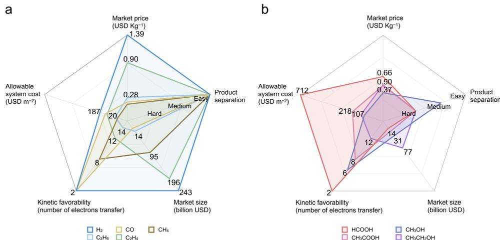
Fig. 4 Economic comparison of common products obtained from solar-driven CO<sub>2</sub>RR. (a) Gaseous products and (b) liquid products.
