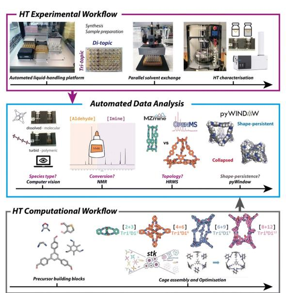
Fig. 3 An automated, high-throughput workflow for the synthesis, analysis, and property prediction of POCs. Image reproduced with permission from ref. 60.
