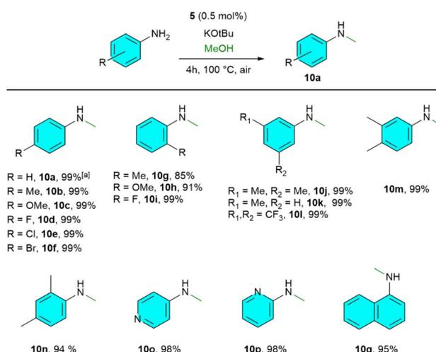
Scheme 2 *N*-methylation of primary aromatic amines. Reaction conditions: amine (1 mmol), methanol (0.2 ml), base (150 mol%), **5** (0.5 mol%) at 100 °C for 4 h under air atmosphere. [a] yields for all *N*-methylated products were obtained from GC-MS analysis using mesitylene as the internal standard.
