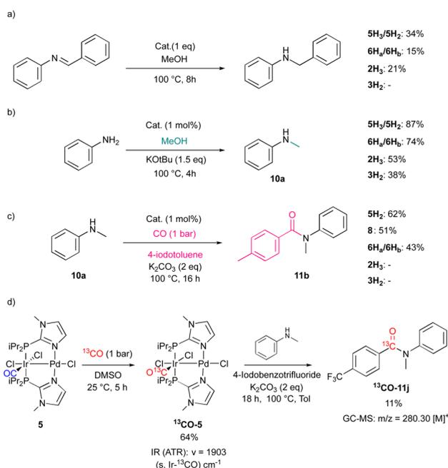
Scheme 5 Model reactivity studies of hydrido or carbonyl complexes; (a) imine bond hydrogenation. (b) *N*-methylation of aniline using hydrido complexes. (c) Aminocarbonylation of **10a**. (d) Reactivity of **5** toward <sup>13</sup>CO and its activity in the aminocarbonylation of *N*-methylaniline.
