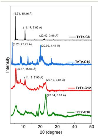
Fig. 5  $\,$  X-ray diffraction pattern of the assembled TzTz derivatives from CHCl $_3$ : ACN composition.
