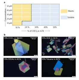
Fig. 2 (a) Concentration-composition phase diagram of TzTz-C8 showing the conditions under which sheets are observed. (b) Representative POM image (under cross-polarizers) of the large-area 2D sheets observed in different solvent combinations ( $c=40~\mu\text{M}$ ).
