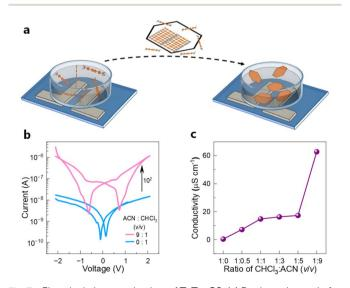
Fig. 7 Electrical characterization of TzTz-C8. (a) Device schematic for the conductivity measurements. (b) Comparison of I-V sweep between TzTz-C8 in pure CHCl<sub>3</sub> and in 10% CHCl<sub>3</sub> in ACN. (c) Comparison of conductivity on increasing the ratio of ACN in the mixture.
