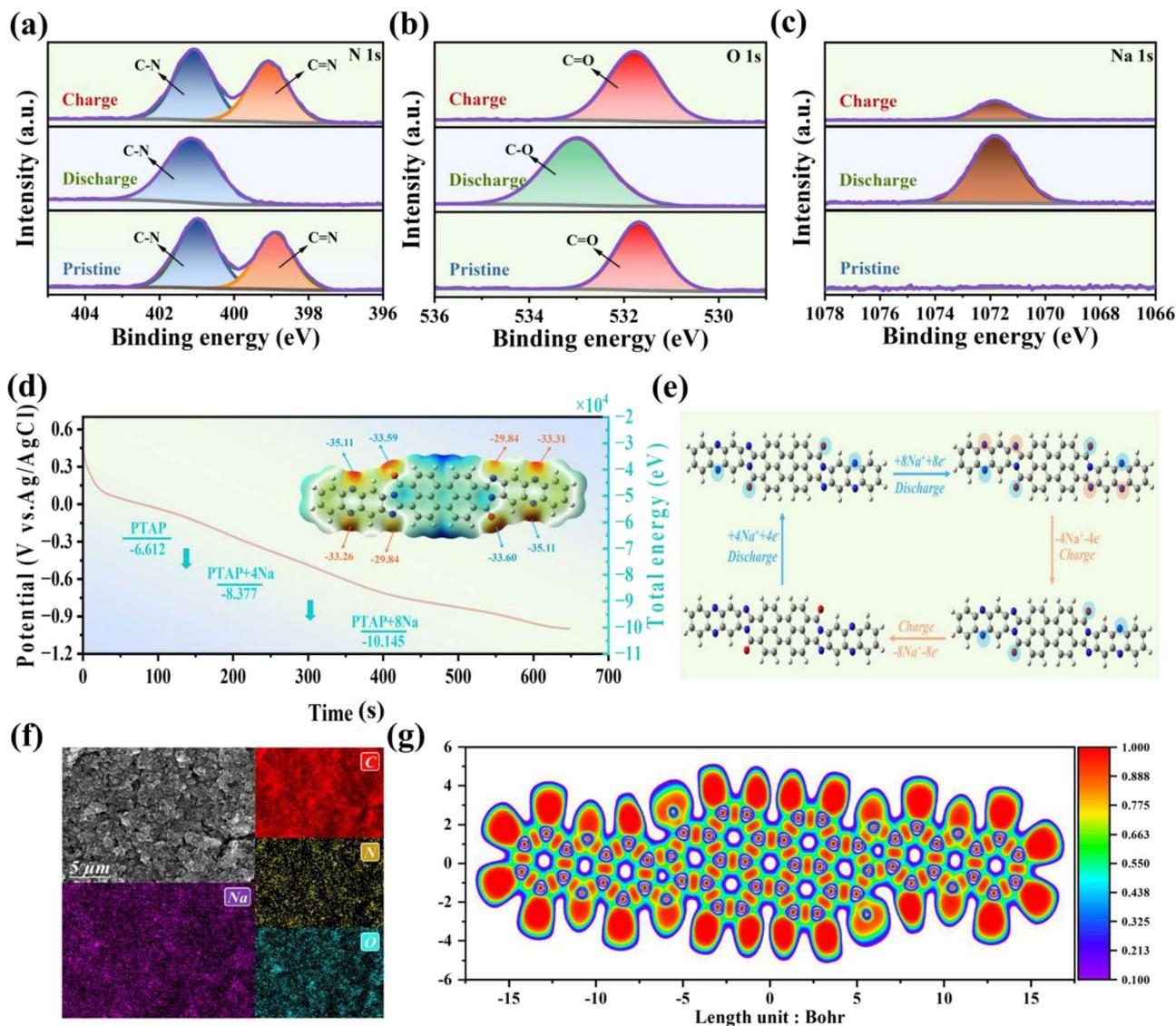
Fig. 4 *Ex situ* XPS spectra of (a) N 1s, (b) O 1s and (c) Na 1s for the PTAP electrode in pristine, fully charged and discharged states. (d) Calculated total energies of sodium-intercalated PTAP structures, indicating stability variations with sodium incorporation, and (e) depicting key electrochemical reactions and ion transport dynamics. (f) SEM image and the corresponding EDS mapping images at the adsorption state. (g) The corresponding ELF image of a PTAP molecule.
