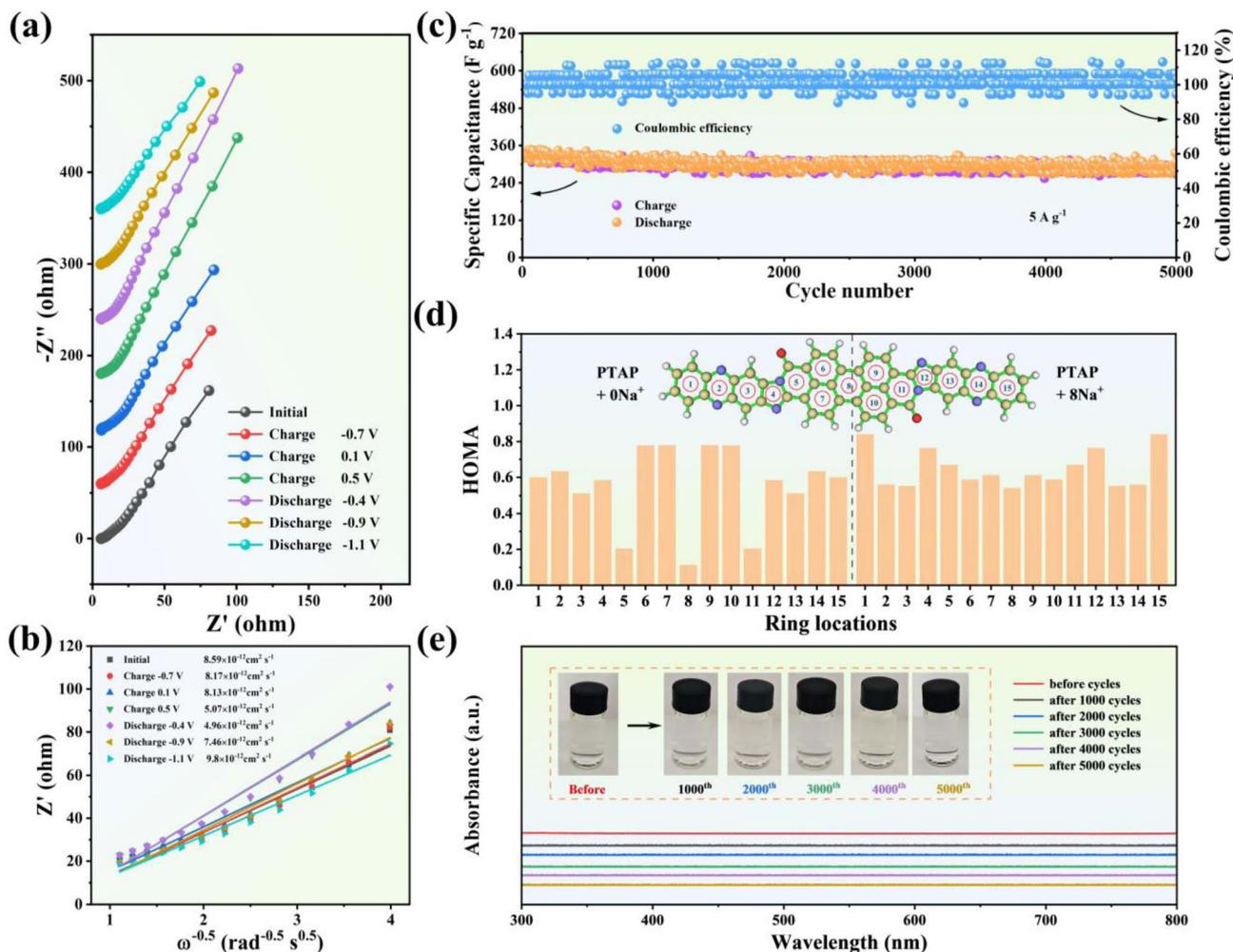
Fig. 3 (a) EIS plots of the PTAP electrode at various discharged/charged states and (b) corresponding  $\text{Na}^+$  diffusion coefficients. (c) Long-term cycling stability of the PTAP electrode over 5000 cycles. (d) The calculated HOMA values for the PTAP molecule before and after complete  $\text{Na}^+$  adsorption. (e) UV-Vis spectra and digital photographs of the electrolyte at different cycles.
