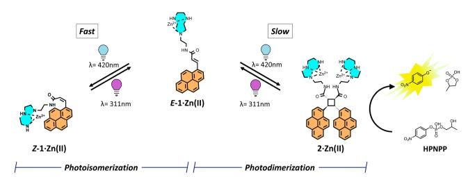
Fig. 1 Reaction scheme highlighting the studied processes: upon irradiation at 420 nm the  $E-1 \cdot \text{Zn}(II)$  monomer can isomerize into  $Z-1 \cdot \text{Zn}(II)$  (fast) or dimerize to give  $2 \cdot \text{Zn}(II)$  (slow). The formed photodimer can catalyze the transphosphorylation of HPNPP into p-nitrophenol (PNP) and cyclic phosphate. The photoinduced processes can be reverted by irradiating with a wavelength of 311 nm.
