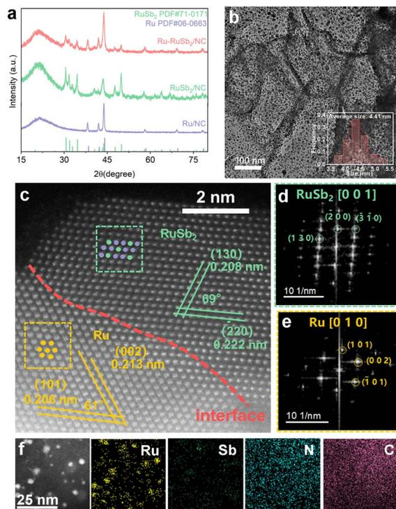
**Fig. 1** (a) The XRD pattern of Ru/NC, Ru–RuSb<sub>2</sub>/NC and RuSb<sub>2</sub>/NC. (b) The TEM image of Ru–RuSb<sub>2</sub>/NC and the corresponding size distribution. (c) The atomic-resolution HAADF-STEM image of Ru–RuSb<sub>2</sub>/NC. The FFT of RuSb<sub>2</sub> (d) and Ru (e) from STEM images of panels (c). (f) HAADF STEM image and corresponding EDX mappings of Ru–RuSb<sub>2</sub>/NC.
