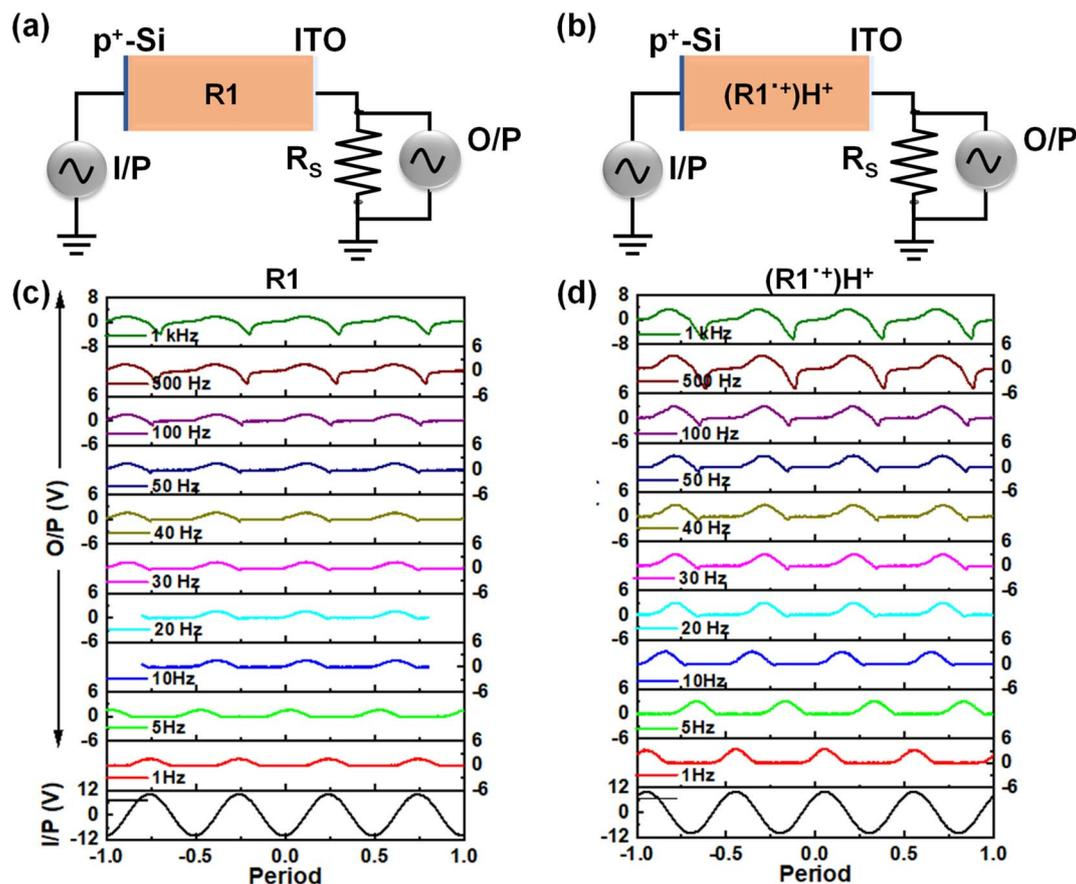
Fig. 4 Investigation of alternating current to direct current conversion efficiency. (a) A measurement setup for AC to DC signal conversion for **R1** and (b)  $(\mathbf{R1}^+)\mathbf{H}^+$ . (c) Conversion of AC to DC signals of  $\text{p}^+\text{-Si}/\mathbf{R1}_{58\text{ nm}}/\text{ITO}$  and (d)  $\text{p}^+\text{-Si}/(\mathbf{R1}^+)\mathbf{H}^+_{58\text{ nm}}/\text{ITO}$  after 60 s of exposure. The data were collected at different frequencies (minimum 1 Hz and maximum 1 kHz).
