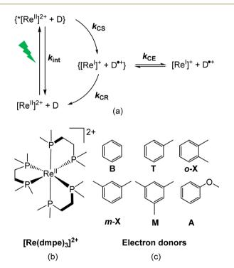
Fig. 1 (a) Schematic reductive photocycle involving a rhenium(II) complex,  $[Re]^{2+}$ , as the photosensitizer and an electron donor (D).  $K_{int}$  = intrinsic decay rate of excited  $[Re]^{2+}$ ;  $k_{CS}$  = rate of CS;  $k_{CR}$  = rate of CR;  $k_{CE}$  = rate of CE. Chemical structure of (b)  $[Re(dmpe)_3]^{2+}$  and (c) the investigated electron donors: benzene (B), toluene (T), o-xylene (o-X), m-xylene (m-X), mesitylene (M), and anisole (A).
