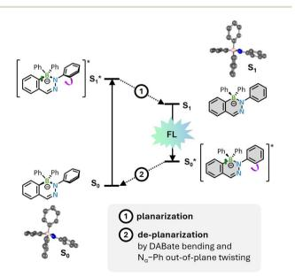
Fig. 6 Schematic depiction of the geometric changes during the excitation and relaxation of the model DABate  $5\text{Ph}^-$  (grey = planarized).
