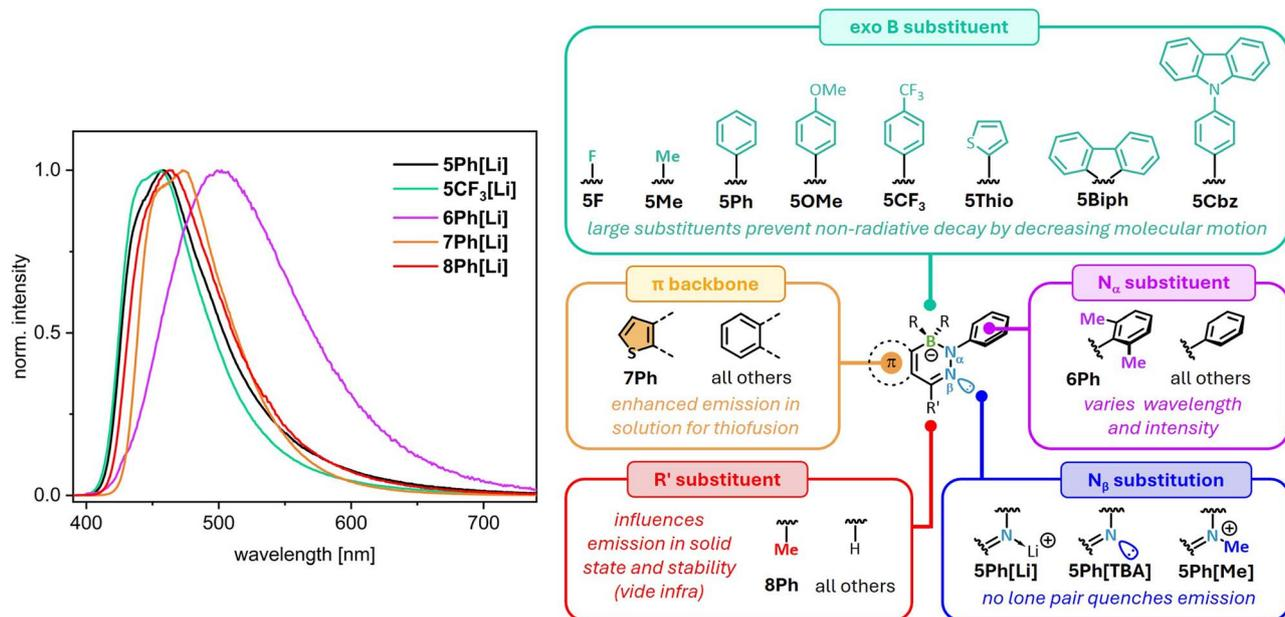
Fig. 3 Normalized emission spectra of 5Ph[Li], 5CF<sub>3</sub>[Li], 6Ph[Li], 7Ph[Li], and 8Ph[Li] in THF. Inset: overview of structural factors influencing emission.
