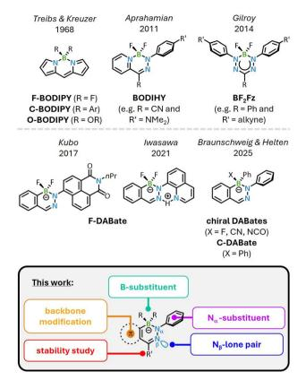
Fig. 1 Basic scaffolds of established BODIPY, BODIHY and BF₂Fz dyes (top), diazaborinates (DABates, middle) and investigated structure–properties relationships in this work (bottom).
