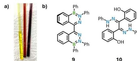
Fig. 8 (a) NMR samples of a DABate before (left, yellow solution) and after (middle and right, red solutions) atmosphere exposure. (b) Compounds **9** and **10** crystallized as part of the decomposition studies (for XRD structures see ESI, appendix Fig. S107 and S108<sup>†</sup>).
