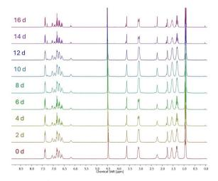
Fig. 9 Stacked  $^1$ H NMR spectra of **8Ph[TBA]** in a 1:1  $D_2O/THF-d_8$  mixture under air over a period of 16 d, showing no significant decomposition.
