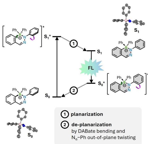
**Fig. 6** Schematic depiction of the geometric changes during the excitation and relaxation of the model DABate **5Ph<sup>-</sup>** (grey = planarized).
