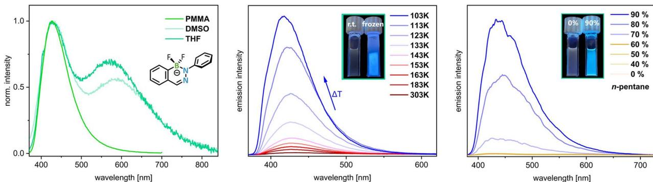
Fig. 4 Emission spectra of 5F[TBA] in different solvents (left), variable-temperature emission spectra of 5F[TBA] in 2-MeTHF from 303 to 103 K (middle), and emission spectra of 5F[TBA] in THF/*n*-pentane mixtures (conc.  $5 \times 10^{-5}$  M). Inset: structure of the compound and corresponding samples under UV light.
