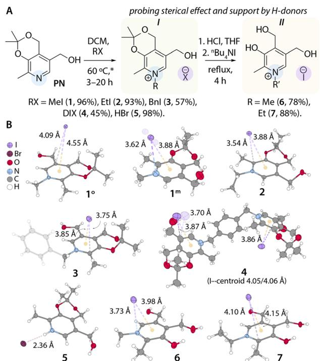
Fig. 2 (A) Synthesis of pyridinium salts 1–7: \* in a sealed tube and (B) molecular structures of ion pairs 1–7 (displacement ellipsoids are shown at the 50% probability level) with depicted shortest I $\cdots$ C, I $\cdots$ N, and I $\cdots$ centroid distances.
