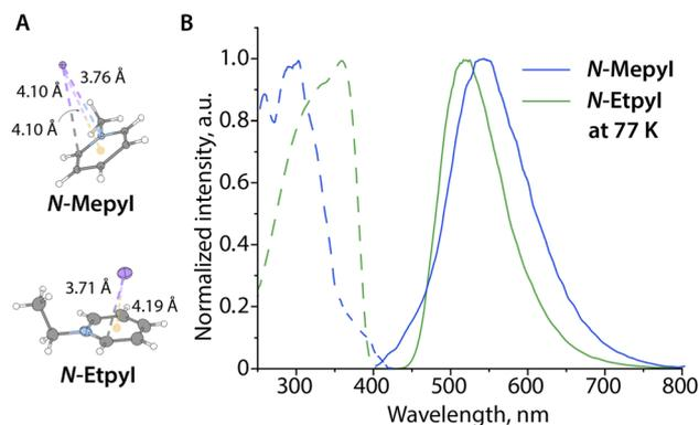
Fig. 1 (A) Molecular structures of ion pairs **N-Mepyl** (ball and stick representation) and **N-Etpyl** (displacement ellipsoids are shown at the 50% probability level) with depicted shortest anion- $\pi$  interactions, and (B) their excitation (dashed) and emission (solid) spectra measured from solids at 77 K.
