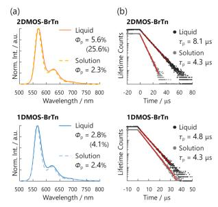
Fig. 3 Steady-state photoluminescence (PL) spectra (a) and PL decay curves (b) of 2DMOS-BrTn (top) and 1DMOS-BrTn (bottom) in solution (1.0  $\times$   $10^{-5}$  M in cyclohexane) and solvent-free liquid state, evaluated at room temperature in air. Red lines in panel b denote the fit to the curve.  $\Phi_{\rm p}$ , RTP quantum yields;  $\tau_{\rm p}$ , phosphorescence lifetimes. Values in parentheses are  $\Phi_{\rm p}$  evaluated under Ar.
