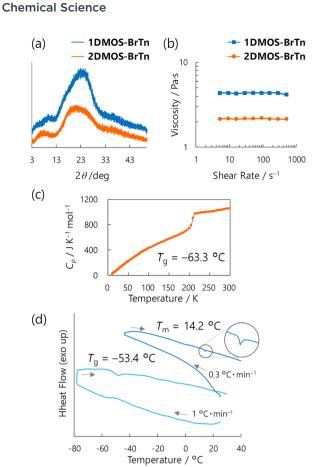
Fig. 2 (a) X-ray diffraction profiles of diketones. (b) Steady-flow viscosity of diketones as a function of shear rate. (c) Temperature dependence of heat capacity of 2DMOS-BrTn. (d) Temperature dependence of differential scanning calorimetry of 1DMOS-BrTn.
