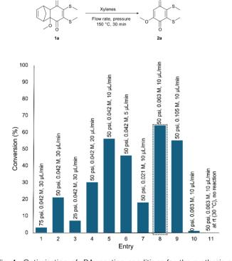
Fig. 4 Optimization of rDA reaction conditions for the synthesis of blue venom compound (best condition boxed).
