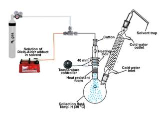
Fig. 3 Schematic diagram of microdroplet setup.
