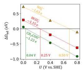
Fig. 2 Adsorption grand free energy ( $\Delta \Omega_{ad}$ ) versus applied potential (U on the SHE scale) for  $SO_4^{2-}$ ,  $HCO_3^{-}$ , and  $CH_3COO^-$  adsorbed on Pt(111). The labeled slopes and x-intercept of fitted linear lines represent  $\gamma$  (unit e) and  $U^0$  (unit V), respectively.
