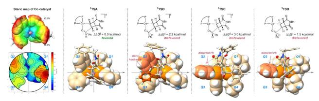
Scheme 6 DFT calculations for stereo-determining transition states. A topographic steric map of the Co catalyst as well as transition states with different configurations is depicted. 4f used in experiments was employed in our calculations.
