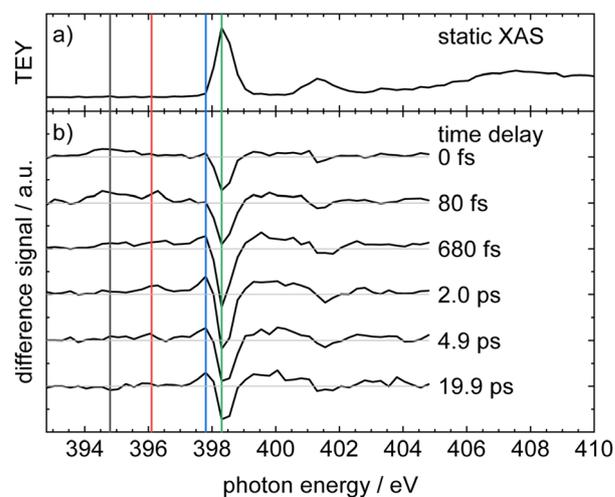
Fig. 3 Experimental X-ray absorption spectra of phenanthridine measured as total electron yield (TEY): (a) static XAS and (b)  $\Delta XAS$  at different pump-probe delay times. Vertical lines indicate probe photon energies where delay traces were recorded.
