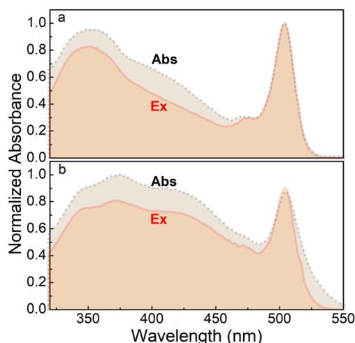
Fig. 3 Overlay of excitation (solid, red – Ex) and absorption (dash dot, black – Abs) spectra of (a) T4F3BDP and (b) F3T4BDP in toluene ( $\lambda_{\text{em}} = 517 \text{ nm}$ ). The excitation spectra were corrected for the instrument response function and were normalized with respect to the absorption spectra at 517 nm.
