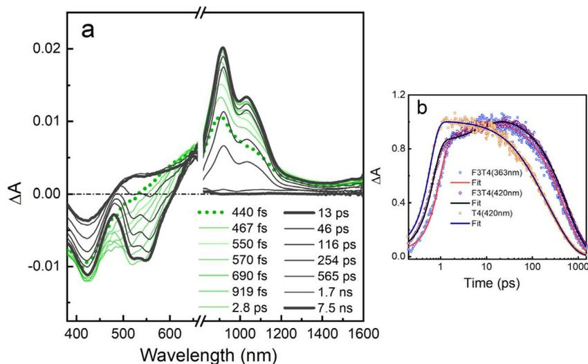
Fig. 5 (a) Femtosecond TA spectra of **F3T4** in toluene solvent with excitation at 363 nm. Delay times range from 440 fs to 7.5 ns, see legend inset for time labels. (b) TA kinetics at 919 nm for **T4** ( $\lambda_{\text{ex}} = 420$  nm), **F3T4** ( $\lambda_{\text{ex}} = 363$  nm) and **F3T4** ( $\lambda_{\text{ex}} = 420$  nm). Evolution associated difference spectra (EADS) obtained from global analysis of data is provided in Fig. S60 in SI.
