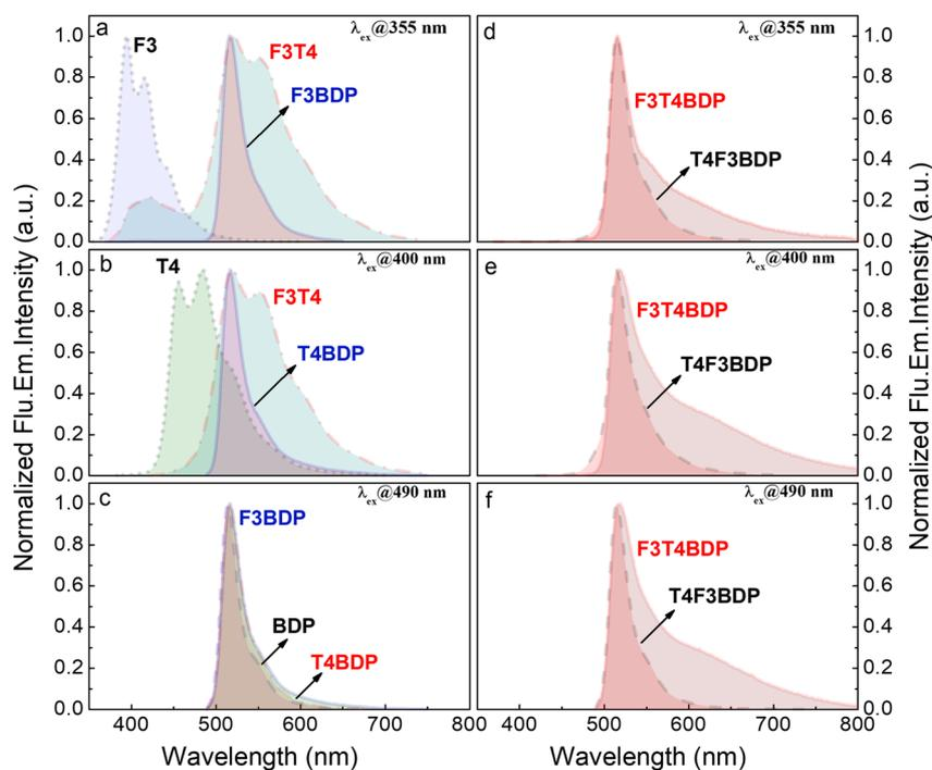
Fig. 2 Normalized fluorescence spectra of oligomers in toluene solution. (a) F3, F3T4 and F3BDP,  $\lambda_{\text{ex}} = 355$  nm. (b) T4, F3T4 and T4BDP,  $\lambda_{\text{ex}} = 400$  nm. (c) F3BDP, T4BDP and BDP,  $\lambda_{\text{ex}} = 490$  nm. (d) F3T4BDP and T4F3BDP,  $\lambda_{\text{ex}} = 355$  nm. (e) F3T4BDP and T4F3BDP,  $\lambda_{\text{ex}} = 400$  nm. (f) F3T4BDP and T4F3BDP,  $\lambda_{\text{ex}} = 490$  nm.
