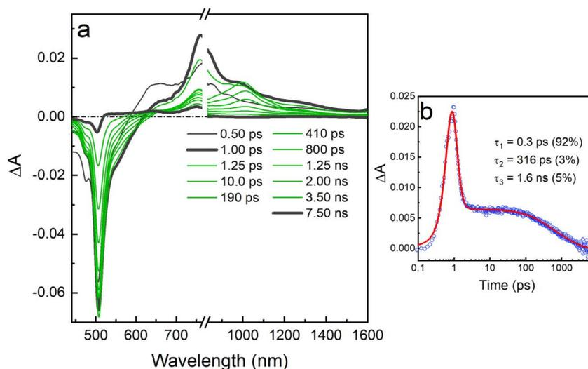
Fig. 4 Femtosecond TA difference spectra of **T4BDP** in toluene solution with excitation at 420 nm. (a) Visible-near-infrared spectra as a function of delay time ranging from 500 fs to 7.5 ns. (b) TA kinetics at 841 nm, symbols show the experimental data and solid line is fit with parameters shown in inset. Evolution associated difference spectra (EADS) obtained from global analysis of data is provided in Fig. S59 in SI.
