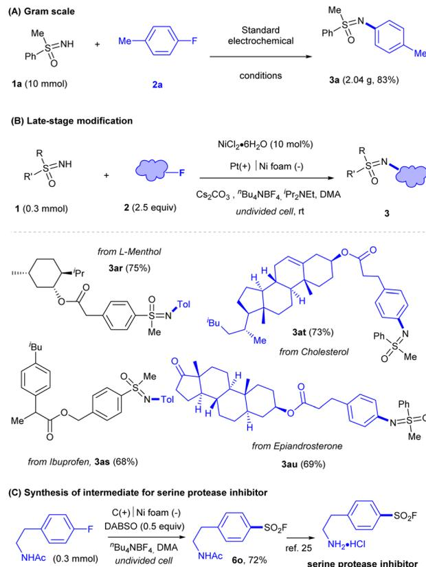
Fig. 4 Synthetic applications. Reaction conditions for late-stage modification: **1** (0.30 mmol), **2** (0.75 mmol),  $\text{NiCl}_2 \cdot 6\text{H}_2\text{O}$  (10 mol%),  $\text{Cs}_2\text{CO}_3$  (2.0 equiv.),  ${}^i\text{Pr}_2\text{NEt}$  (1.5 equiv.),  ${}^t\text{Bu}_4\text{NBF}_4$  (1.0 equiv.), DMA (4 mL) in an undivided cell at rt under an argon atmosphere. For details, please see the ESI.†
