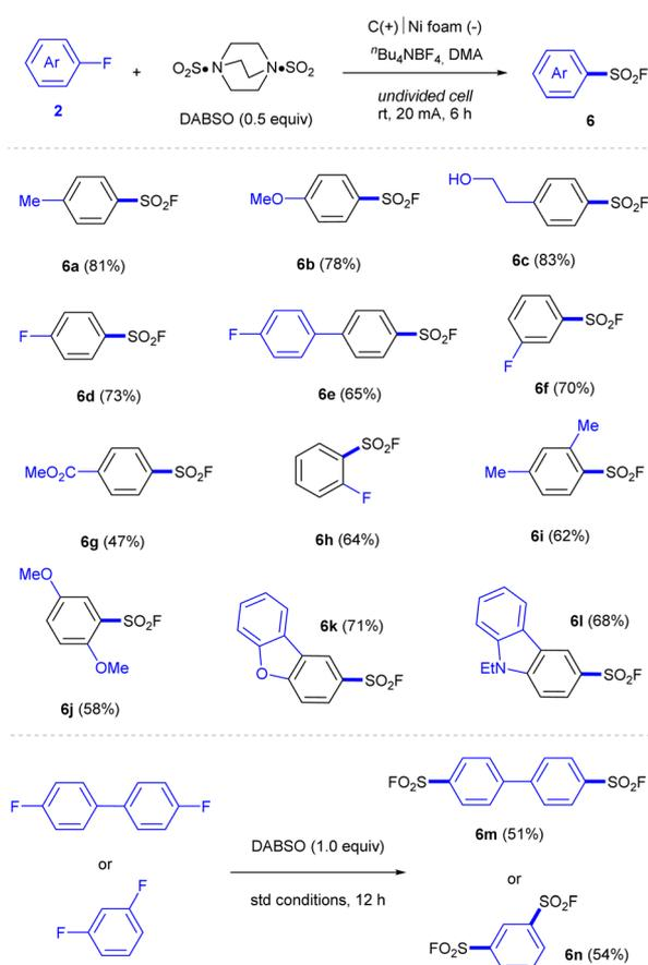
Fig. 3 Fluorosulfonylation with aryl fluorides. Reaction conditions: **2** (0.3 mmol), DABSO (0.15 mmol),  ${}^t\text{Bu}_4\text{NBF}_4$  (1.0 equiv.), DMA (4 mL) in an undivided cell, 20 mA, 6 h, argon. For details, please see the ESI.†
