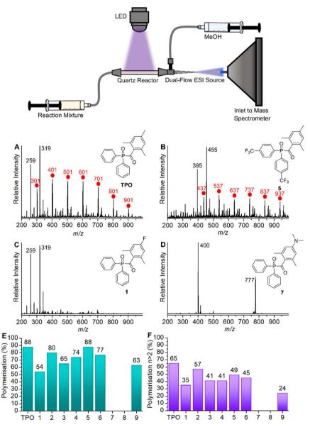
Fig. 2 (Top) Schematic of the quartz cell photochemical reactor setup. Representative mass spectra from the reaction of MMA with (A) TPO. (B) MAPO 5. (C) MAPO 1. (D) MAPO 7. (E) Polymerisation percentages of MMA with each MAPO in this study. (F) Polymerisation percentages of MMA with each MAPO in this study, where n > 2.
