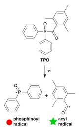
Scheme 1 Photolysis of TPO through Norrish type I cleavage to produce the phosphinoyl and acyl radicals. Coloured symbols are assigned for clarity in later discussion.
