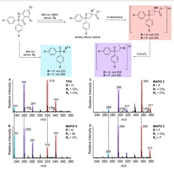
Fig. 5 Scheme (Top) – the proposed oxygenated byproducts generated from the reaction of MAPOs with MMA at 395 nm. (Bottom) – Mass spectra at m/z 320–380 of the reaction of MMA with (A) TPO, (B) MAPO 9, (C) MAPO 2, and (D) MAPO 3.
