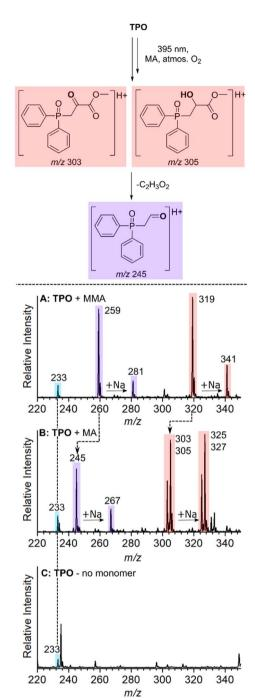
Fig. 6 Scheme (Top) – the proposed oxygenated byproducts generated from the reaction of MAPOs with MA at 395 nm. (Bottom) – Mass spectra at m/z 220–340 of the reaction of TPO with (A) MMA, (B) MA, and (C) no monomer (MeOH was used as the solvent where no monomer was used).
