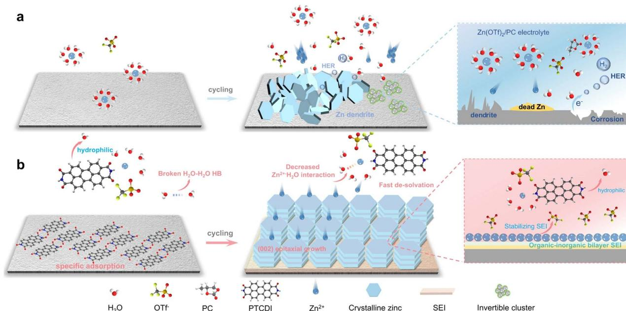
**Scheme 1** Schematic illustration of the Zn surface evolution. (a) Schematic diagram of Zn dendrites and HER in Zn(OTf)<sub>2</sub>/PC electrolyte. (b) The mechanism for enhancing zinc electrode stability by PTCDI additive.
