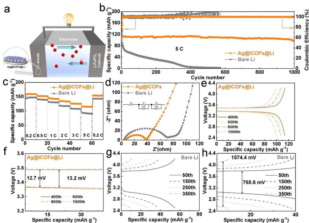
Fig. 6 (a) Schematic diagram of a full battery. Electrochemical performance of Li@Ag@ICOFs|LFP and bare Li|LFP full cells at (b) 5C and (c) different rates. (d) Electrochemical impedance spectra of full cells after 100 cycles. (e) Charge–discharge profiles of Li@Ag@ICOFs|LFP full cells at different cycling numbers and (f) enlarged profiles. (g) Charge–discharge profiles of bare Li|LFP full cells and (h) enlarged profiles.
