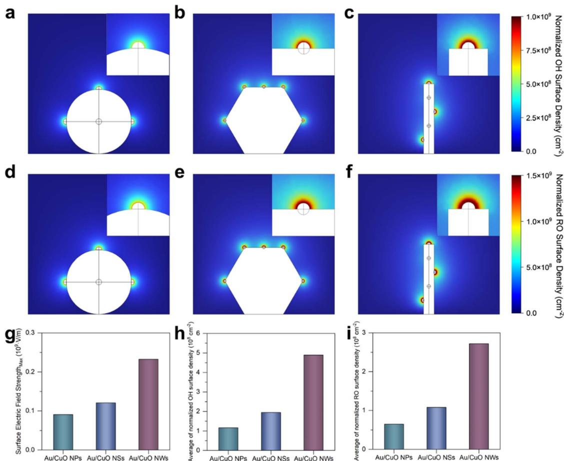
Fig. 4 Simulated normalised OH<sup>-</sup> surface density distribution on (a) Au/CuO NPs, (b) Au/CuO NSs and (c) Au/CuO NWs. Simulated distribution of normalised benzyl alkoxide (RO) surface density on (d) Au/CuO NPs, (e) Au/CuO NSs and (f) Au/CuO NWs. (g) The maximum surface electric field strength of three Au/CuO catalysts. (h) The average of normalised OH<sup>-</sup> surface density on three Au/CuO catalysts. (i) The average of normalised RO surface density on three Au/CuO catalysts.
