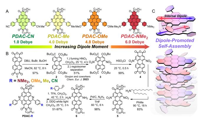
Fig. 1 Synthesis and assembly of PDACs with tunable  $\mu_g$ . (A) Series of increasing internal dipole moments in PDAC molecules: PDAC-CN green, PDAC-Me yellow, PDAC-OMe Orange, PDAC-NMe<sub>2</sub> red. Dipoles were calculated using Multiwfn program (see Section E in ESI†). (B) Synthetic approach to prepare annullatively extended PDACs with various permanent dipoles. (C) Cartoon depiction of PDAC supramolecular assembly.
