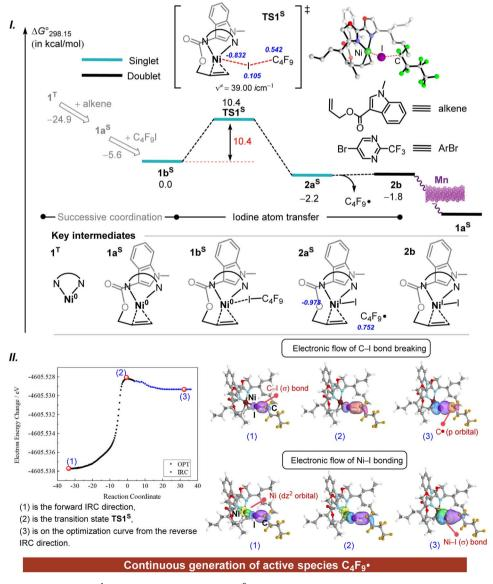
Fig. 2 Gibbs energy profile (in kcal  $mol^{-1}$ ) of radical initiation by the  $Ni^0$  catalyst (I). IBO analysis of the open-shell singlet process in iodine atom transfer (II). Blue bold italic text represents spin density values, and red numbers indicate Gibbs activation energies for the corresponding steps.
