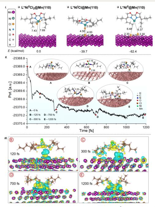
Fig. 1 Thermodynamic evaluation (I), potential energy landscape of heterogeneous reduction of Ni<sup>II</sup>Cl<sub>2</sub> by the Mn(110) surface (II), and charge density difference between two phases during the reduction process (III) (isovalue = 0.002 e Bohr<sup>-3</sup>).
