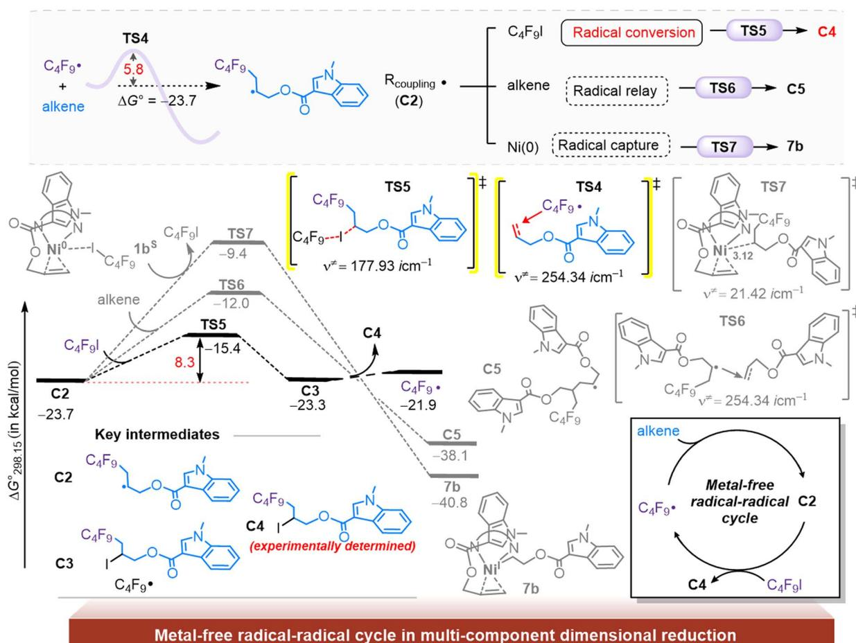
Fig. 3 Gibbs energy profile (in kcal mol<sup>-1</sup>) of polymerization and termination of radicals to form a two-component coupled intermediate C4. Red numbers indicate Gibbs activation energies for the corresponding steps, and the fluorescent yellow line marks the most favorable pathway.
