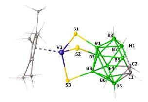
Fig. 7 Molecular structure and labelling diagram of 5. Selected bond lengths (Å) and bond angles (°): V1-S1 2.2194(16), V1-S3 2.2099(15), B3-S3 1.859(6), B1-B8 1.780(9), C1-C2 1.555(8), C2-B7 1.596(8), B8-Hb 1.15(2), B9-Hb 1.16(2), V1-S1-B1 81.01(19), V1-S3-B3 79.42(17), B7-B8-B9 101.7(5), C1-C2-B7 114.3(5).
