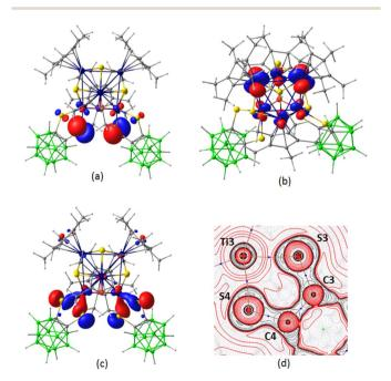
Fig. 2 (a) HOMO, (b) LUMO, and (c) HOMO-13 of 1 (isocontour values:  $\pm 0.045$  [e bohr<sup>-3</sup>]<sup>1/2</sup>). (d) Contour-line diagram of the Laplacian of the electron density along the Ti3-S3-S4 plane in 1.
