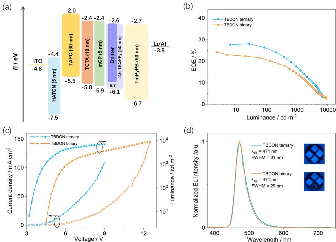
Fig. 6 (a) Device configuration and energy levels for each layer; (b) EQE versus electroluminescence characteristics. (c)  $J$ - $V$ - $L$  characteristics; (d) electroluminescence spectra for devices; inset: images of working devices.
