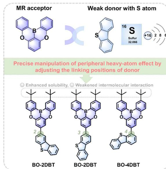
Fig. 1 Schematic illustration of pure violet emitter design strategy by combining DBT with an MR-type acceptor.
