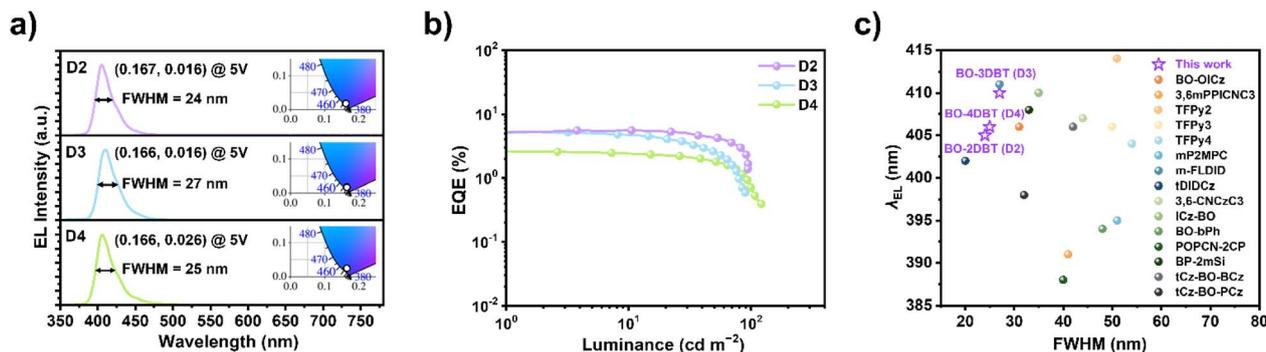
Fig. 5 (a) EL spectra of OLEDs at 5 V. Inset, corresponding CIE image. (b) EQE versus luminance curves. (c) EL peak wavelength versus FWHM of the reported representative violet OLEDs.
