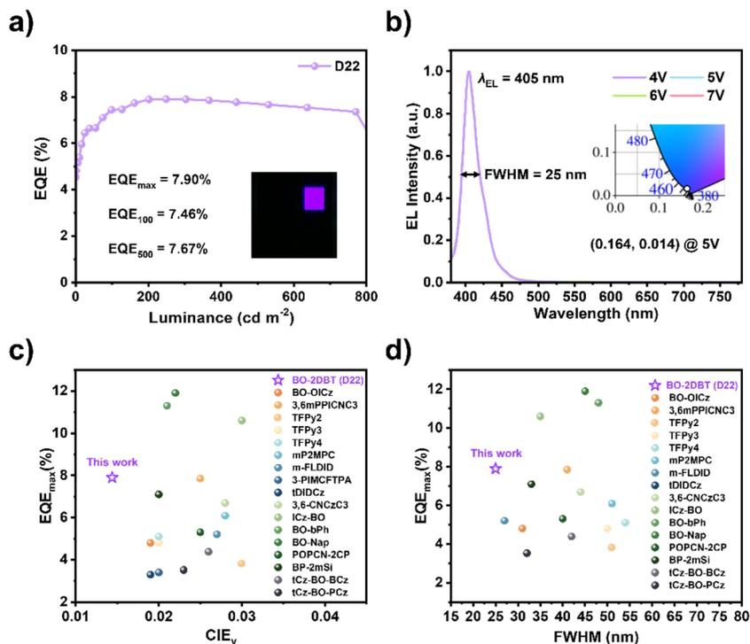
Fig. 6 (a) EQE versus luminance curves. Inset, corresponding light-emitting device. (b) EL spectra of OLEDs at different voltages. Inset, corresponding CIE image. (c)  $\text{EQE}_{\text{max}}$  versus  $\text{CIE}_y$  of the reported representative violet OLEDs ( $\text{CIE}_y \leq 0.03$ ). (d)  $\text{EQE}_{\text{max}}$  versus FWHM of the reported representative violet OLEDs.
