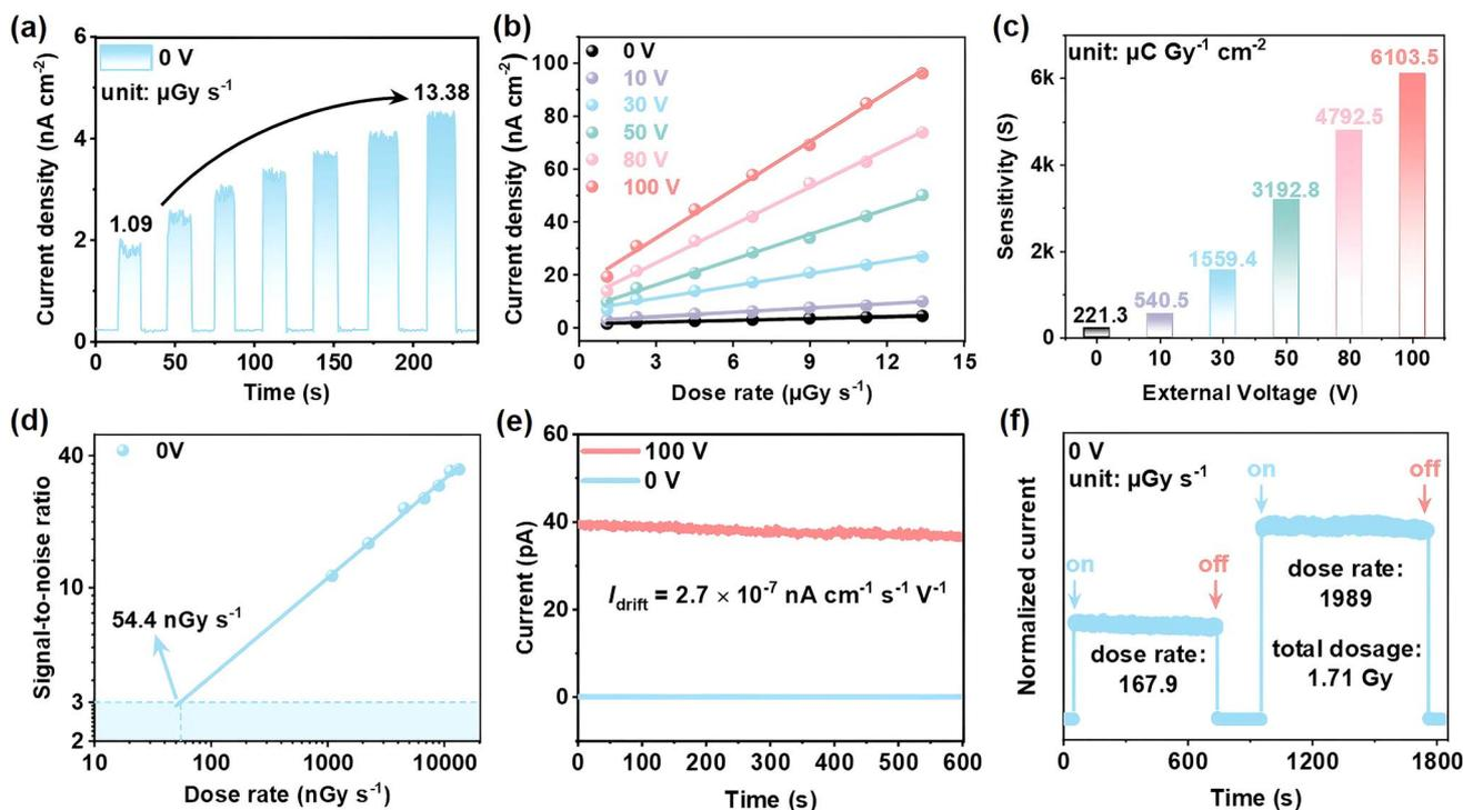
Fig. 3 (a) The current density–time curve of device **1** under 0 V bias as the X-ray radiation dose increases. (b and c) Fitting to obtain the X-ray detection sensitivity of device **1** under different bias voltages. (d) The signal-to-noise ratio (SNR) of device **1** under 0 V bias. (e) Dark current drift of device **1** under 0 V and 100 V bias voltage, respectively. (f) Response stability of device **1** under different high X-ray dose rate irradiation conditions for a long time.
