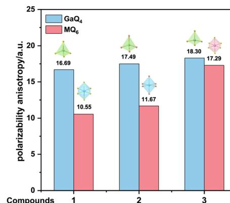
Fig. 3 Polarizability anisotropy of  $\text{GaQ}_4$  tetrahedra and  $\text{MQ}_6$  ( $Q = \text{S}, \text{Se}$ ;  $M = \text{Sc}, \text{In}$ ) tetrahedra.
