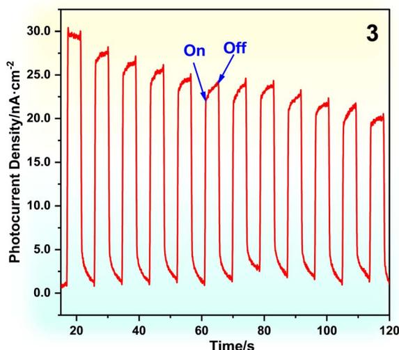
Fig. 4 Photocurrent response curve of 3 (from 15 to 120 seconds).
