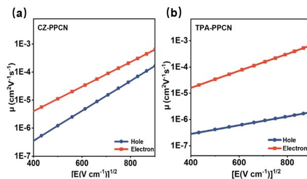
Fig. 4 Charge mobilities *versus* electric field curves for (a) CZ-PPCN and (b) TPA-PPCN. Configuration of the hole-only device: ITO/HATCN (20 nm)/EML (80 nm)/HATCN (20 nm)/Al (100 nm). Configuration of the electron-only device: ITO/LiF (1 nm)/TPBi (10 nm)/EML (80 nm)/LiF (1 nm)/Al (100 nm).
