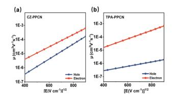
Fig. 4 Charge mobilities *versus* electric field curves for (a) CZ-PPCN and (b) TPA-PPCN. Configuration of the hole-only device: ITO/HATCN (20 nm)/EML (80 nm)/HATCN (20 nm)/Al (100 nm). Configuration of the electron-only device: ITO/LiF (1 nm)/TPBi (10 nm)/EML (80 nm)/LiF (1 nm)/Al (100 nm).
