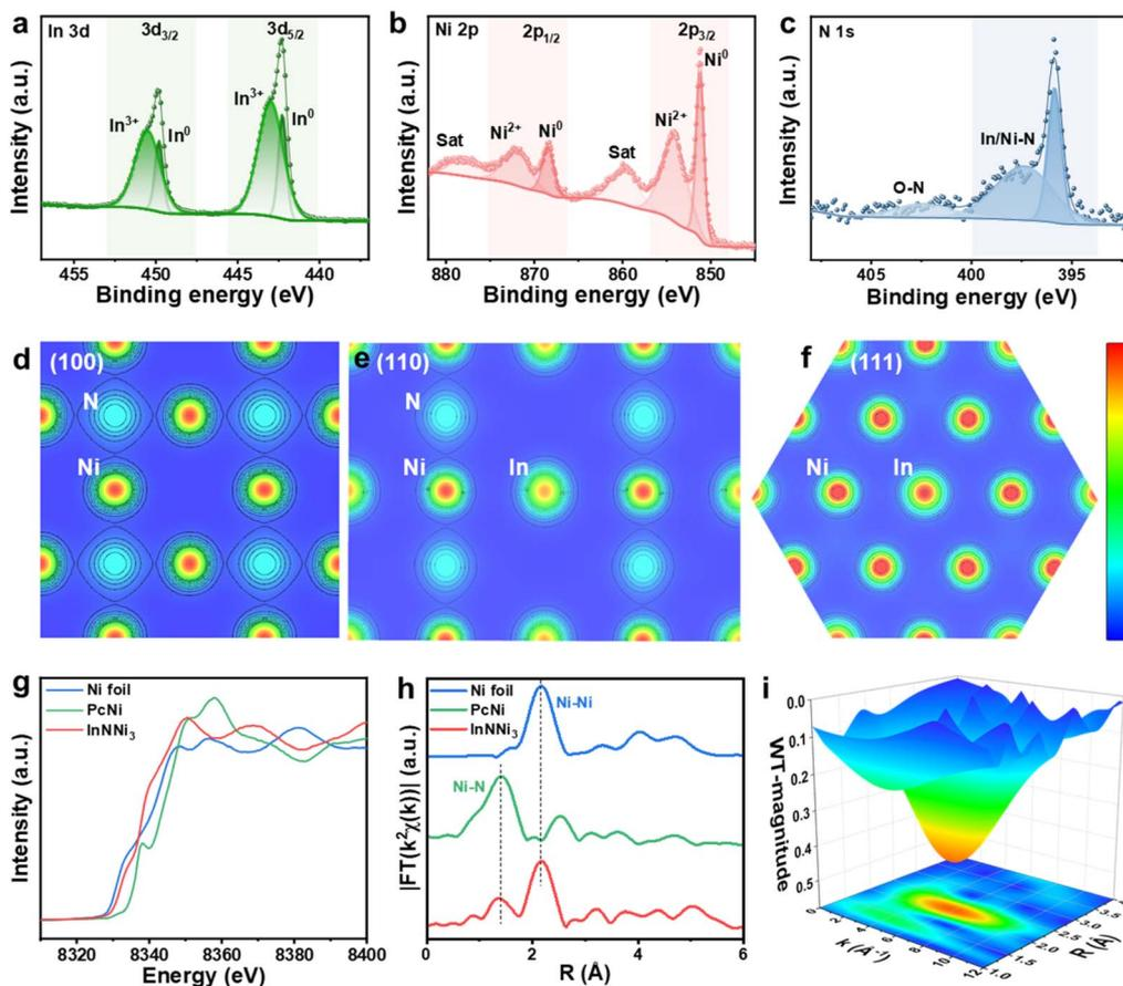
Fig. 2 Surface chemical state, charge density distribution and local coordination of InNNi<sub>3</sub> antiperovskite. XPS spectra: (a) In 3d, (b) Ni 2p and (c) N 1s. Charge density isosurface at different crystal facets: (d) (100), (e) (110), and (f) (111). (g) Ni K-edge XANES spectra. (h) Magnitude of Fourier transformed Ni K-edge EXAFS data. (i) WT-EXAFS signal at the Ni K-edge.
