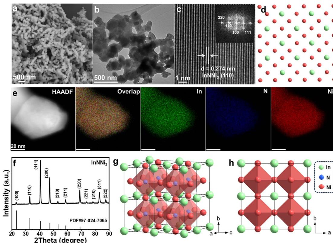
Fig. 1 Morphology, surface and crystal structure characterization of InNNi<sub>3</sub>. (a) SEM image. (b) TEM image. (c) HRTEM image (inset shows the FFT of the corresponding HRTEM area). (d) Simulated atomic models viewed from the same direction as images in panel (c) (In: cyan; Ni: red). (e) HAADF-STEM and EDS mapping images of In/N/Ni elements. (f) Powder XRD patterns. (g and h) Crystal structure viewed from different directions.
