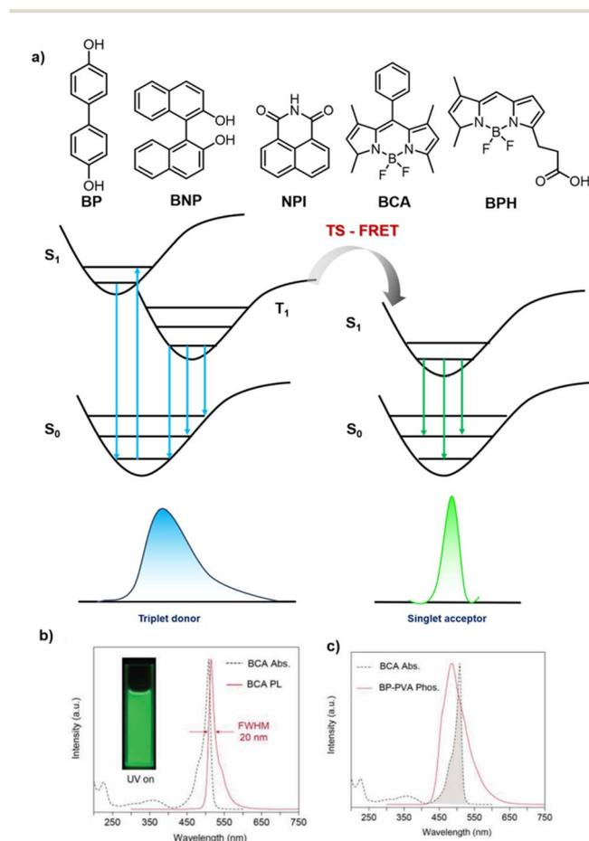
Fig. 10 Narrow-band emitters *via* TS-FRET. (a) Molecular structures of donors (BP, BNP, and NPI) and acceptors (BCA and BPH) and a simplified Jablonski diagram showing the TS-FRET process to produce narrow-band emission. (b) Emission and absorption spectra of acceptor BCA. (c) Spectral overlap of emission of BP (donor) embedded in PVA, and absorption of BCA (acceptor). Adapted with permission from ref. 27a copyright © 2023 Wiley-VCH GmbH.
