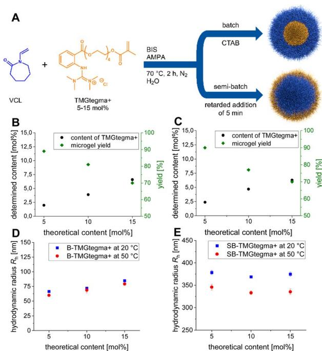
**Fig. 1** (A) Schematic synthesis of guanidine-modified microgels *via* batch and semi-batch precipitation polymerization. Gravimetrically calculated yields and TMGtegma+ contents of the B-TMGtegma+ (B) and SB-TMGtegma+ (C) microgels determined *via*  $^1\text{H}$  NMR spectroscopy. Hydrodynamic radii of the B-TMGtegma+ (D) and SB-TMGtegma+ (E) microgels in methanol at 20 and 50 °C measured *via* DLS.
