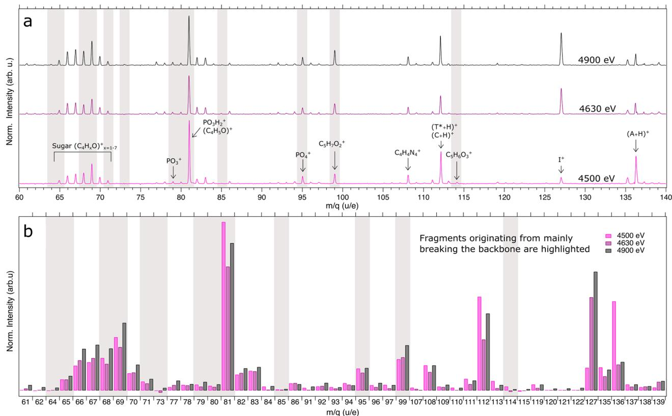
Fig. 5 (a) Measured mass spectrum for AT\*C for three incident photon energies at 4500, 4630 and 4900 eV within the mass range of  $m/q$  60–150. Peaks that contribute to the breakage of the sugar-phosphate backbone are emphasized in gray. (b) Integrated areas of the main peaks from the spectra above.
