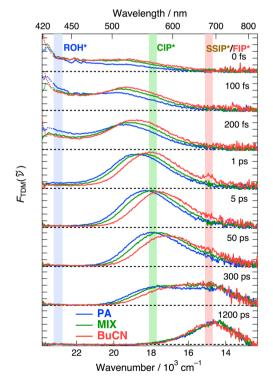
Fig. 3 Time-resolved fluorescence spectra of  $C_4$ -dHONI in the presence of NMI ( $c=200\,\text{mM}$ ) in PA (blue), MIX (green) and BuCN (red). All sub-panels have the identical vertical scale. The colored vertical fills indicate the monitoring ranges for the respective species indicated in the top panel.
