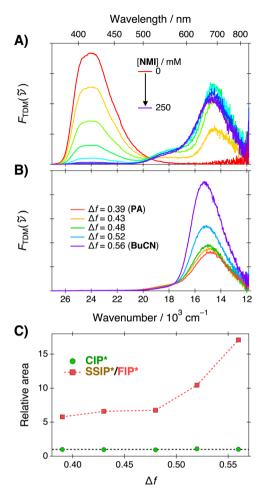
Fig. 2 (A) Steady-state fluorescence spectra of C<sub>4</sub>-dHONI ( $c=13~\mu\text{M}$ ) upon addition of NMI in PA and (B) the spectra in all solvent mixtures in the presence of NMI (c=250~mM). (C) Relative areas of CIP\* and SSIP\*/FIP\* fluorescence bands normalized to mean CIP\* area across all solvent systems.
