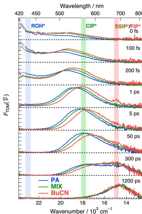
Fig. 3 Time-resolved fluorescence spectra of C<sub>4</sub>-dHONI in the presence of NMI (c = 200 mM) in PA (blue), MIX (green) and BuCN (red). All sub-panels have the identical vertical scale. The colored vertical fills indicate the monitoring ranges for the respective species indicated in the top panel.
