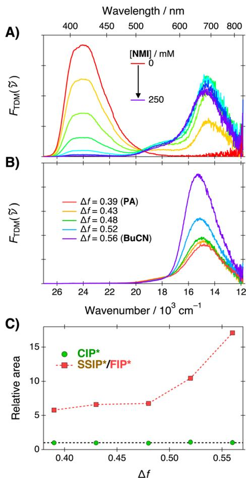
Fig. 2 (A) Steady-state fluorescence spectra of C<sub>4</sub>-dHONI (c = 13 μM) upon addition of NMI in PA and (B) the spectra in all solvent mixtures in the presence of NMI (c = 250 mM). (C) Relative areas of CIP\* and SSIP\*/FIP\* fluorescence bands normalized to mean CIP\* area across all solvent systems.
