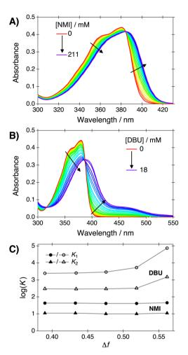
Fig. 1 Steady-state absorption spectra of  $C_4$ -dHONI ( $c = 30 \mu M$ ) upon addition of (A) NMI and (B) DBU in a PA/BuCN solvent mixture ( $\Delta f =$ 0.48). (C) Logarithmic association or deprotonation constants with NMI (solid markers) and DBU (empty markers) in all mixtures as a function of  $\Delta f$ . The lines serve as a guide to the eye. Adapted from ref. 48
