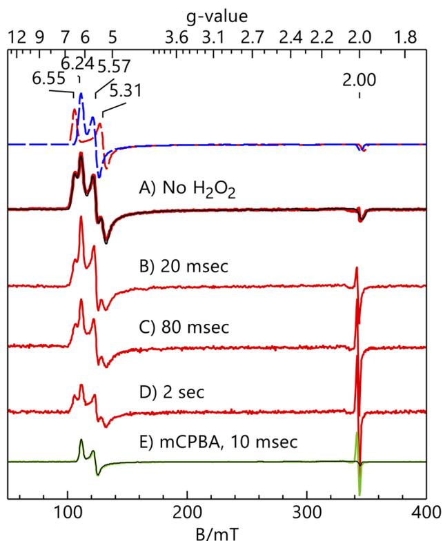
Fig. 5 X-band (9.624 GHz) EPR spectra (red traces) of as-isolated cyt  $c'_\beta$  (A) reacted with  $\text{H}_2\text{O}_2$  (B–D) or mCPBA (green trace, E) at 4 °C and frozen (95 K) at the times listed. All recorded at 11 K and 0.2 mW microwave power. The simulation (black line) overlaid on the data of (A) is the sum of two species in equal amounts:  $E/D = 0.014$  (blue dash),  $E/D = 0.026$  (red dash).
