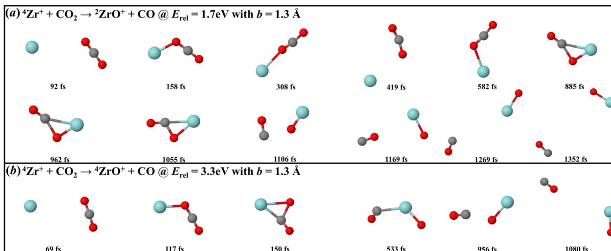
Fig. 4 Exemplary trajectories for the spin-changing channel (ISC) at  $E_{\text{rel}} = 1.7$  eV (a) and spin-conserving channel (SCC) at  $E_{\text{rel}} = 3.3$  eV (b) each for an impact parameter of  $b = 1.3$  Å. Selection is such that only the dominant channel is shown. Full movies can be found in the SI (zirconium = blue, carbon = grey, oxygen = red).
