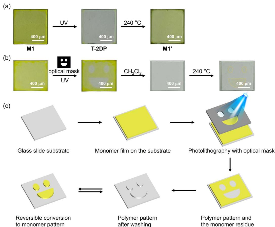
Fig. 4 (a) Photographs of the photo/thermal reversibility behavior of the **M1**/**T-2DP** films on the glass slide substrate. (b) Photographs of the photo/thermal reversible photolithography of the **M1**/**T-2DP** films on the glass slide substrate. (c) Schematic illustration of the photo/thermal reversible photolithography of the **M1**/**T-2DP** film on the glass slide substrate.
