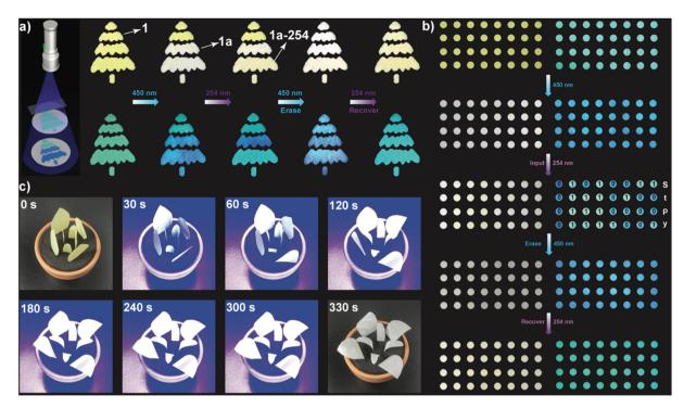
Fig. 5 (a) Schematic illustration of reversible anti-counterfeiting. (b) Optical logic system for reversible information encryption and decryption. (c) A handcrafted item mimicking the blooming process of a flower.
