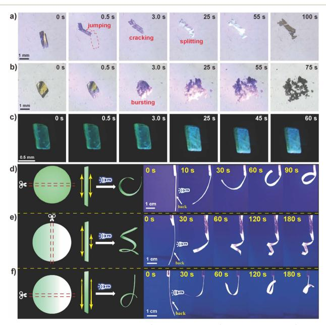
Fig. 4 Digital images of crystal 1 under (a)  $450 \text{ nm} (260 \text{ mW cm}^{-2})$ , (b)  $405 \text{ nm} (260 \text{ mW cm}^{-2})$ , and (c)  $365 \text{ nm} (80 \text{ mW cm}^{-2})$  irradiation with different times. Images of (d) 1-PMMA with uniform distribution, (e) 1-PMMA with a perpendicular concentration gradient, and (f) 1-PMMA with a parallel concentration gradient upon irradiation with 450 nm light.
