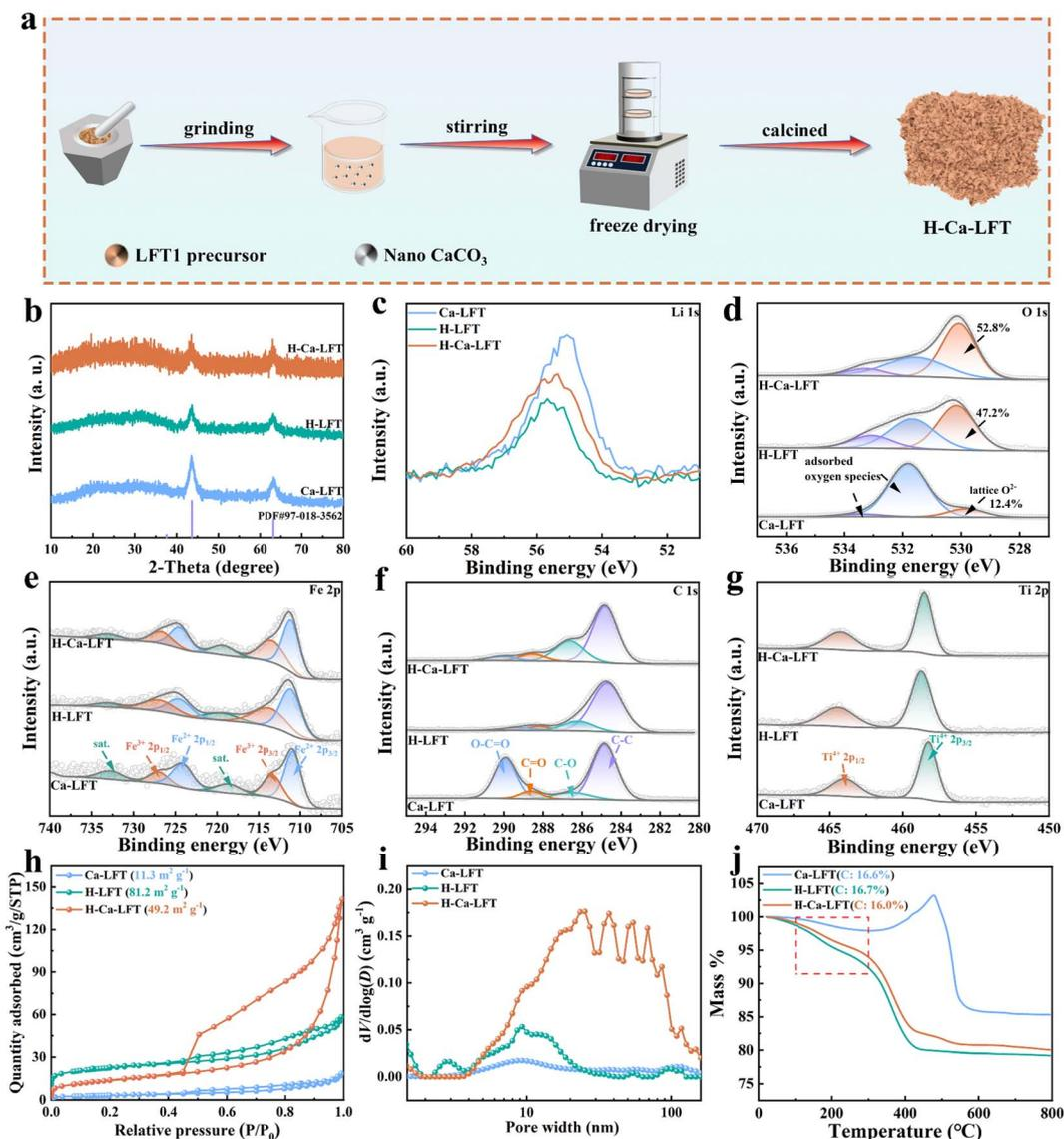
Fig. 1 (a) Schematic diagram of the formation process of H-Ca-LFT, (b) XRD, (c) Li 1s, (d) O 1s, (e) Fe 2p, (f) C 1s, (g) Ti 2p, (h) N<sub>2</sub> adsorption-desorption isotherms, (i) pore size distribution and (j) TG curves of Ca-LFT, H-LFT, and H-Ca-LFT.
