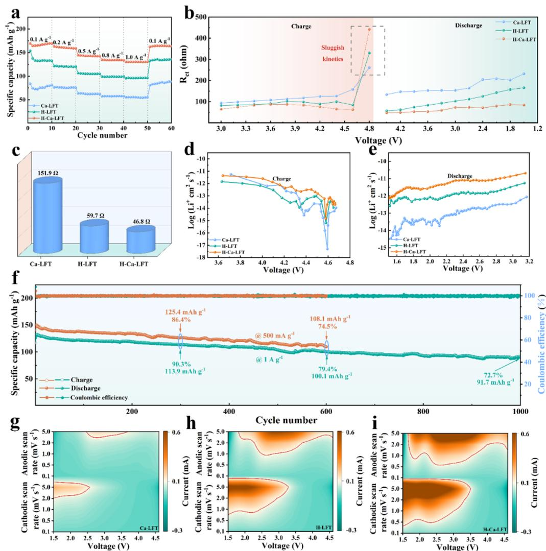
Fig. 4 (a) Rate performances, (b) charge transfer resistance  $R_{ct}$  during the first cycle, (c) interfacial layer resistance  $R_f$ , (d) and (e)  $\text{Li}^+$  diffusion coefficients of Ca-LFT, H-LFT, and H-Ca-LFT, (f) cycling performances at  $500 \text{ mA g}^{-1}$  and  $1.0 \text{ A g}^{-1}$  of H-Ca-LFT, (g–i) contour plots of the CV pattern with different scan rates of Ca-LFT, H-LFT, and H-Ca-LFT.
