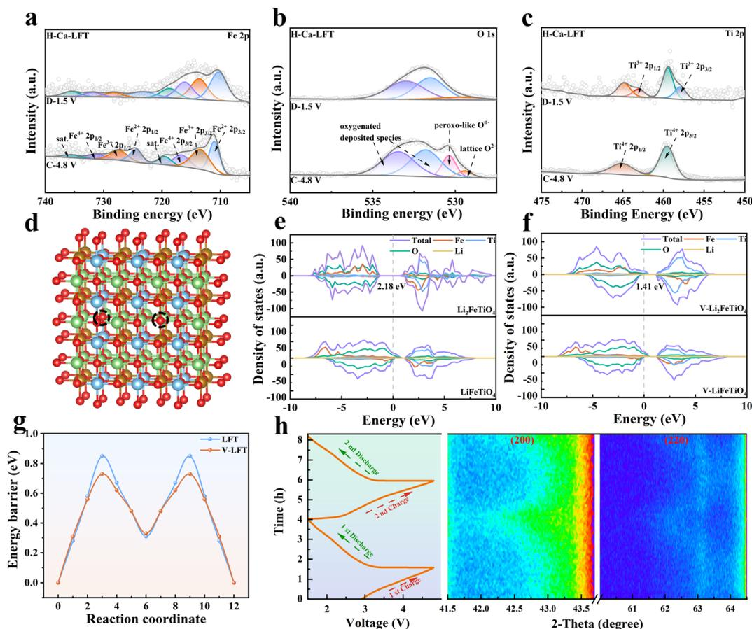
Fig. 5 XPS spectra of (a) Fe 2p, (b) O 1s, and (c) Ti 2p for the H-Ca-LFT electrode at the fully charged and discharged states, (d) crystal structure of V-LFT, (e and f) calculated spin-polarized DOS, (g)  $\text{Li}^+$  diffusion energy barrier for LFT and V-LFT, and (h) voltage profiles and contour plots of *in situ* XRD for H-Ca-LFT.
