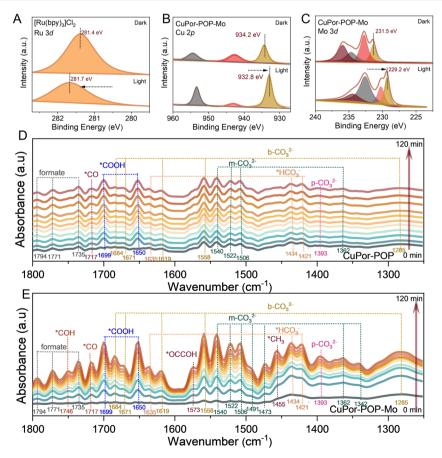
Fig. 4 Quasi-in situ XPS spectra and in situ ATR-FTIR spectra. Quasi-in situ XPS spectra of (A) Ru 3d, (B) Cu 2p and (C) Mo 3d for [Ru(bpy)<sub>3</sub>]Cl<sub>2</sub> and CuPor-POP-Mo under light and in the dark. Room temperature in situ ATR-FTIR spectra of (D) CuPor-POP and (E) CuPor-POP-Mo for the detection of intermediates during CO<sub>2</sub> photoreduction.
