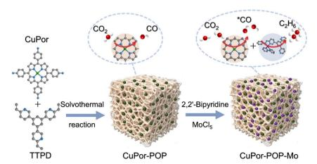
Fig. 1 Schematic illustration for the synthesis of CuPor-POP-Mo and photocatalytic CO<sub>2</sub> reduction. Here, the amine monomer is 5,10,15,20tetrakis(4-aminophenyl)-21H,23H-porphine-Cu(II) (CuPor), and the aldehyde monomer is 5,5',5''-(benzene-1,3,5-triyl)tripicolinaldehyde (TTPD).
