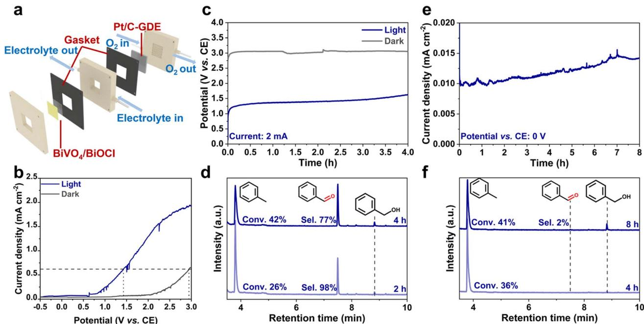
Fig. 5 (a) The layout of the homemade flow cell. (b) LSV curves of the scale-up  $\text{BiVO}_4/\text{BiOCl}$  photoanode in the flow cell. (c) Evolution of the cell potential as a function of time during constant current reaction. (d) GC spectra of the flow cell in a constant current reaction mode with illumination. (e)  $J-t$  curve of the bias-free flow cell without bias. (f) GC spectra of the bias-free flow cell. BD represents benzaldehyde.
