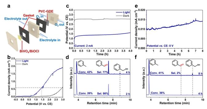
Fig. 5 (a) The layout of the homemade flow cell. (b) LSV curves of the scale-up BiVO<sub>4</sub>/BiOCl photoanode in the flow cell. (c) Evolution of the cell potential as a function of time during constant current reaction. (d) GC spectra of the flow cell in a constant current reaction mode with illumination. (e) J-t curve of the bias-free flow cell without bias. (f) GC spectra of the bias-free flow cell. BD represents benzaldehyde.
