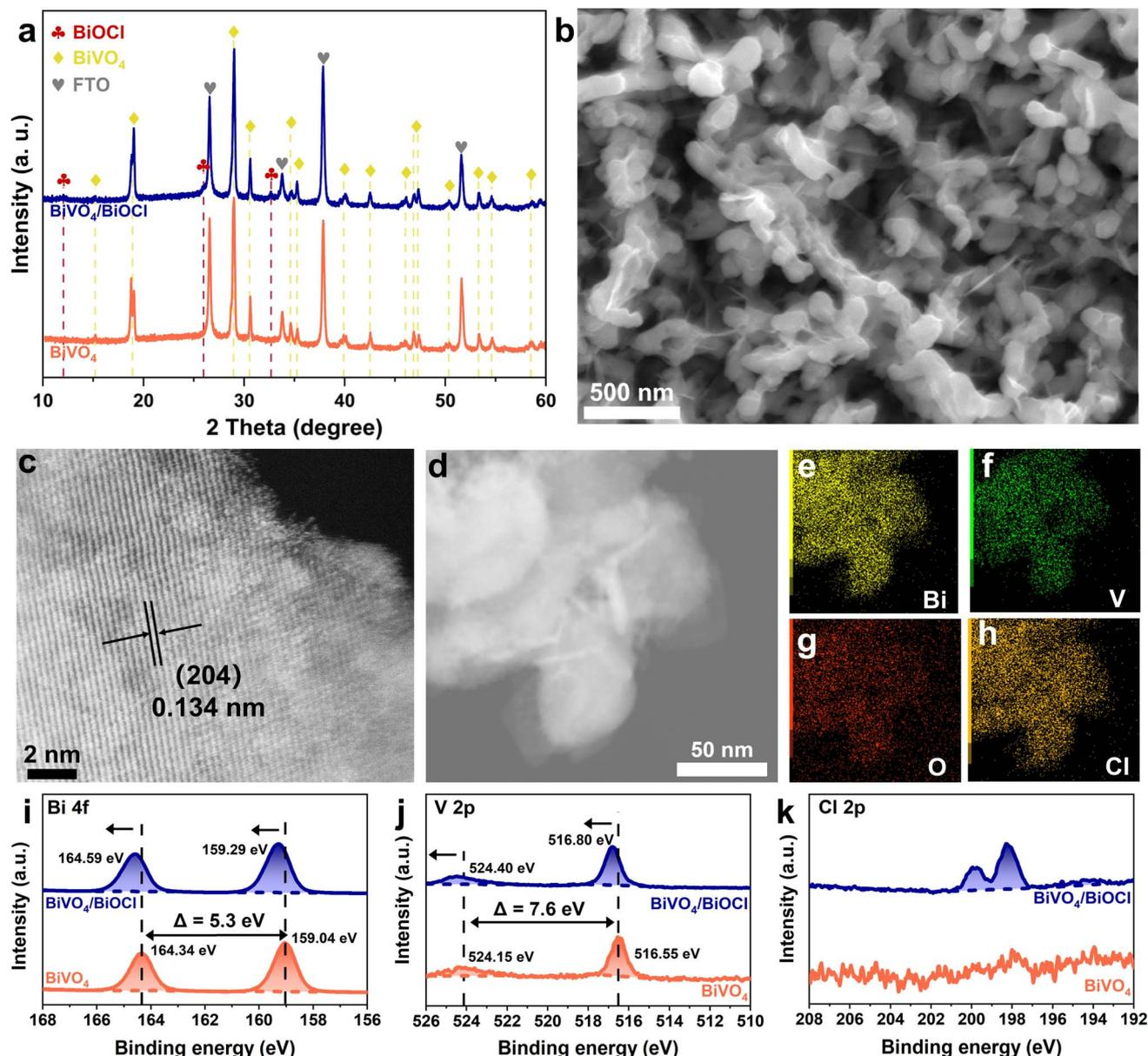
Fig. 1 (a) XRD spectra of  $\text{BiVO}_4$  and  $\text{BiVO}_4/\text{BiOCl}$ . (b) SEM image of  $\text{BiVO}_4/\text{BiOCl}$ . (c) AC-TEM image of  $\text{BiVO}_4/\text{BiOCl}$ . (d) TEM image and (e–h) corresponding EDX mapping images of  $\text{BiVO}_4/\text{BiOCl}$ . (i) XPS Bi 4f spectra, (j) XPS V 2p spectra, and (k) XPS Cl 2p spectra of  $\text{BiVO}_4$  and  $\text{BiVO}_4/\text{BiOCl}$ .
