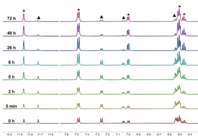
Fig. 2  $^1\text{H}$  NMR spectrum (600 MHz,  $\text{DMSO}-d_6$ , 298 K) of the transformation of  $\text{Na}_4[\text{Si}_2\text{D}_3]$  from helicates ( $\Delta\Delta/\Delta\Delta$ ) to mesocate ( $\Delta\Delta$ ) over time. (▲) represents helicates ( $\Delta\Delta/\Delta\Delta$ ) and \* represents mesocate ( $\Delta\Delta$ ).
